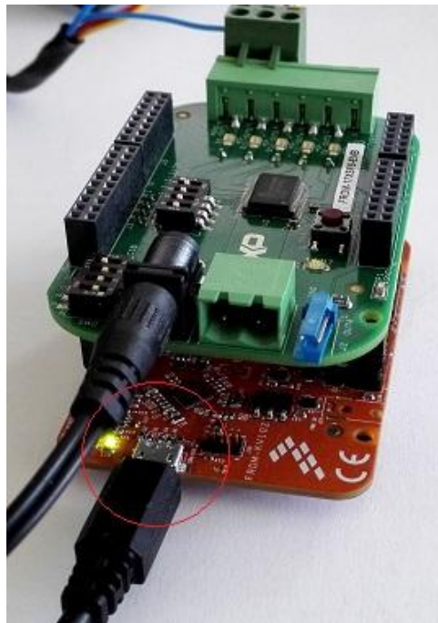
Figure 3 OpenSDA PC-MCU Debug Connection
