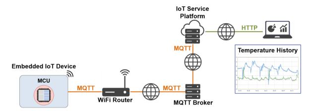
Fig. 1: Unsecured IoT device connecting to the cloud
