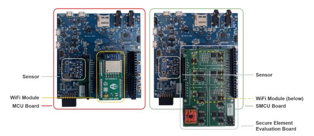
Fig. 7: Unsecured (left) and Secured IoT Device (right)
