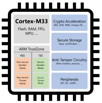
Fig. 5: Secure microcontroller (SMCU)
