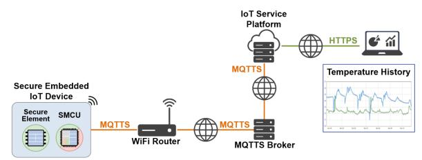
Fig. 6: Secured IoT device connecting to the cloud
