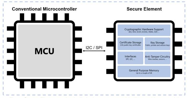
Fig. 4: Secure Element – physically isolate cryptographically sensitive material
