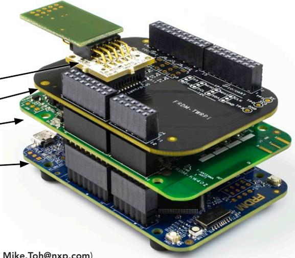
The image shows a stack of four NXP Freedom Board components. From bottom to top, they are: a blue FRDM-K64F board, a green FRDM-KW40Z board, a black FRDM-TWRPI adaptor board, and a green TWRPI-I2C adaptor board. Arrows point from the text labels to each of these boards.
