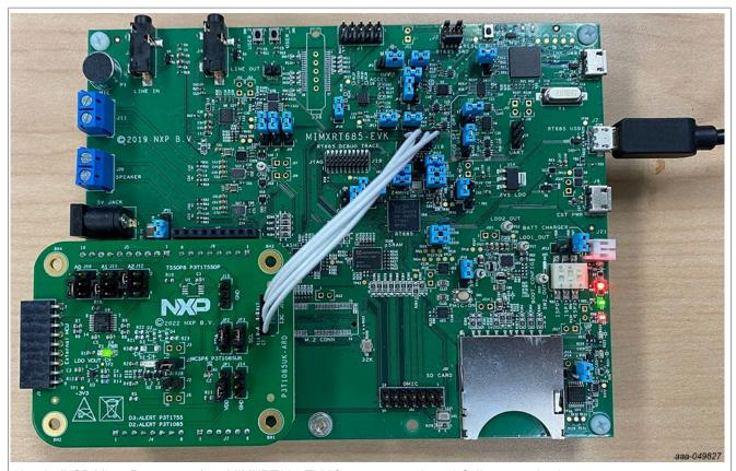
Use J7 (USB Micro-B connector) on MIMXRT685-EVK for power supply and GUI communication port. Figure 3. P3T1085UK-ARD evaluation board connecting to the MIMXRT685-EVK MCU board
