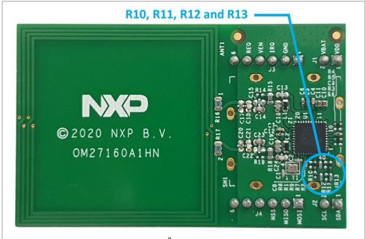
Figure 9. OM27160A1HN NFC controller I<sup>2</sup>C address configuration
