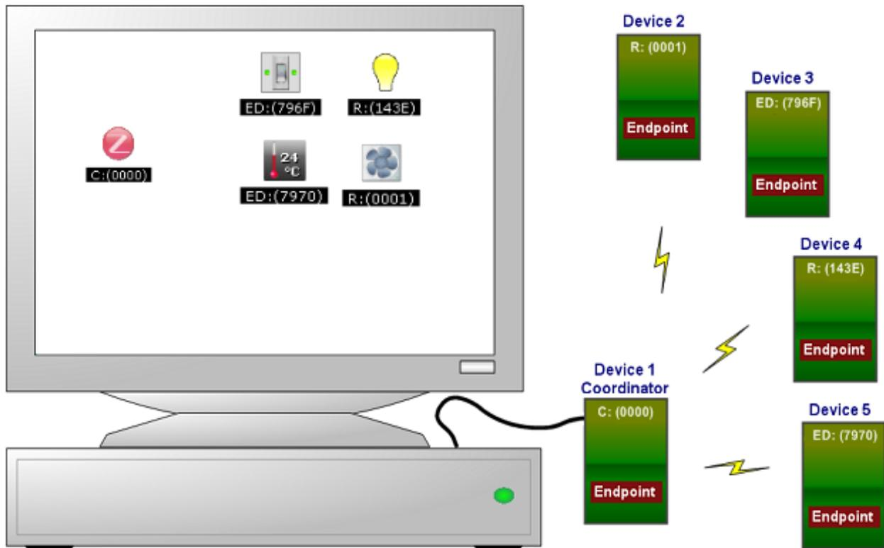
Figure 1-1. Home Automation Setup Example
