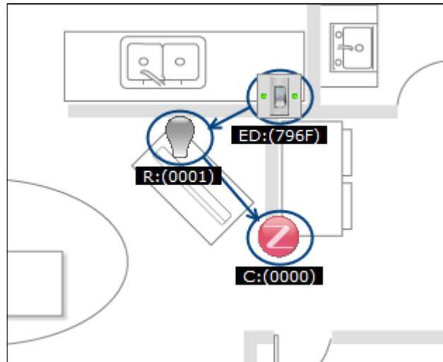
**Figure 4-12. New Binding Made from the On/Off Switch to the On/Off Light**
