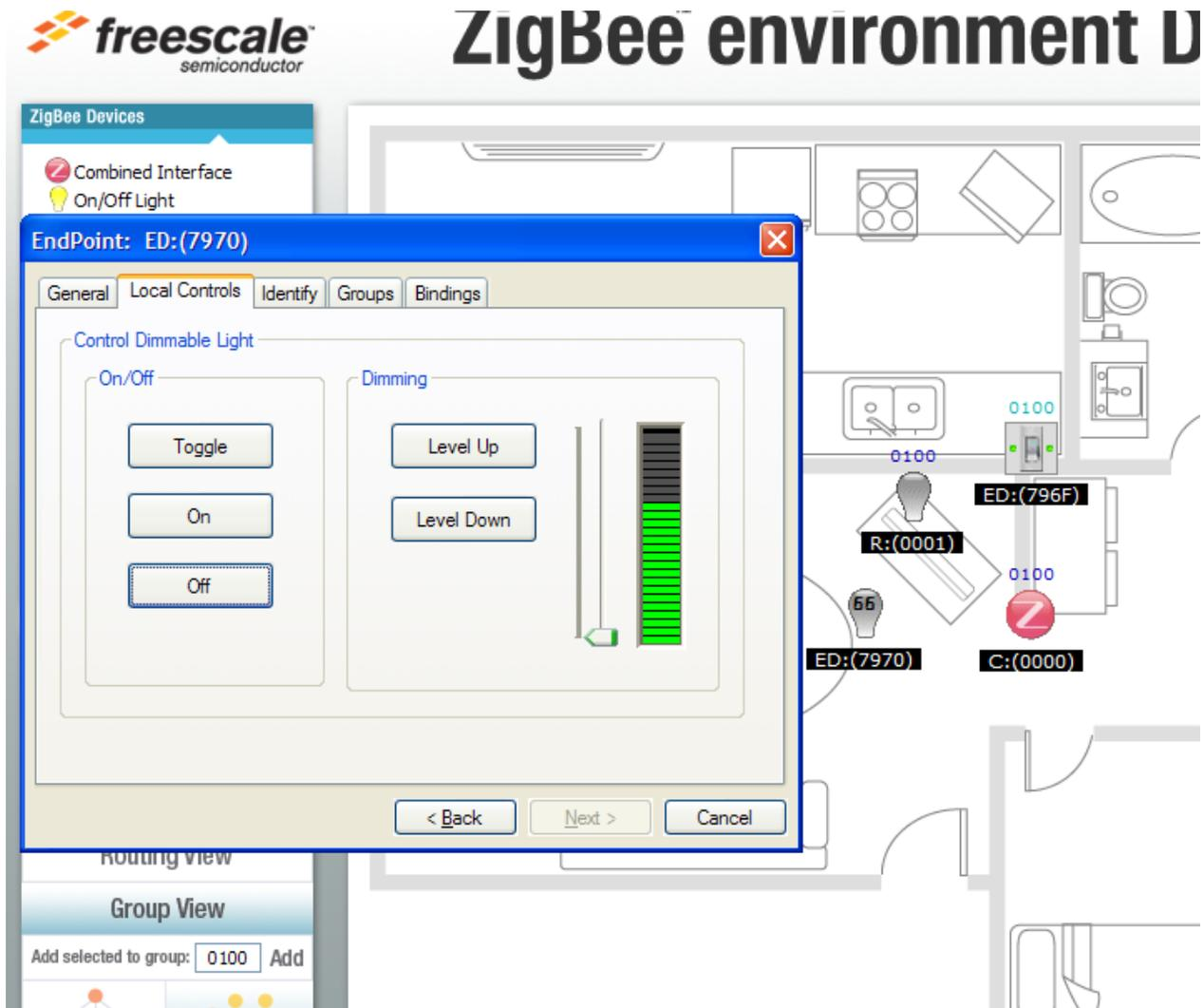
Figure 4-22. Turning Dimmable Light Off
