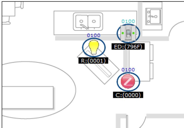
Figure 4-17. ZigBee Nodes Showing their Group IDs and Group IDs for Bindings
