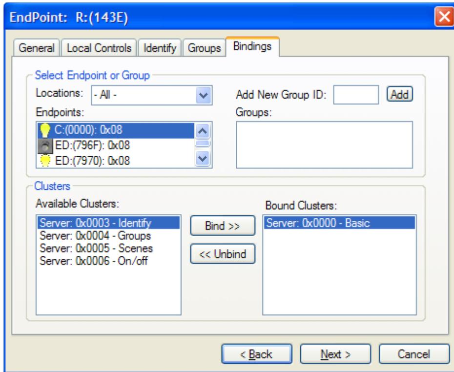
**Figure 7-5. Binding Window with a Binding Made on the Basic Cluster.**
