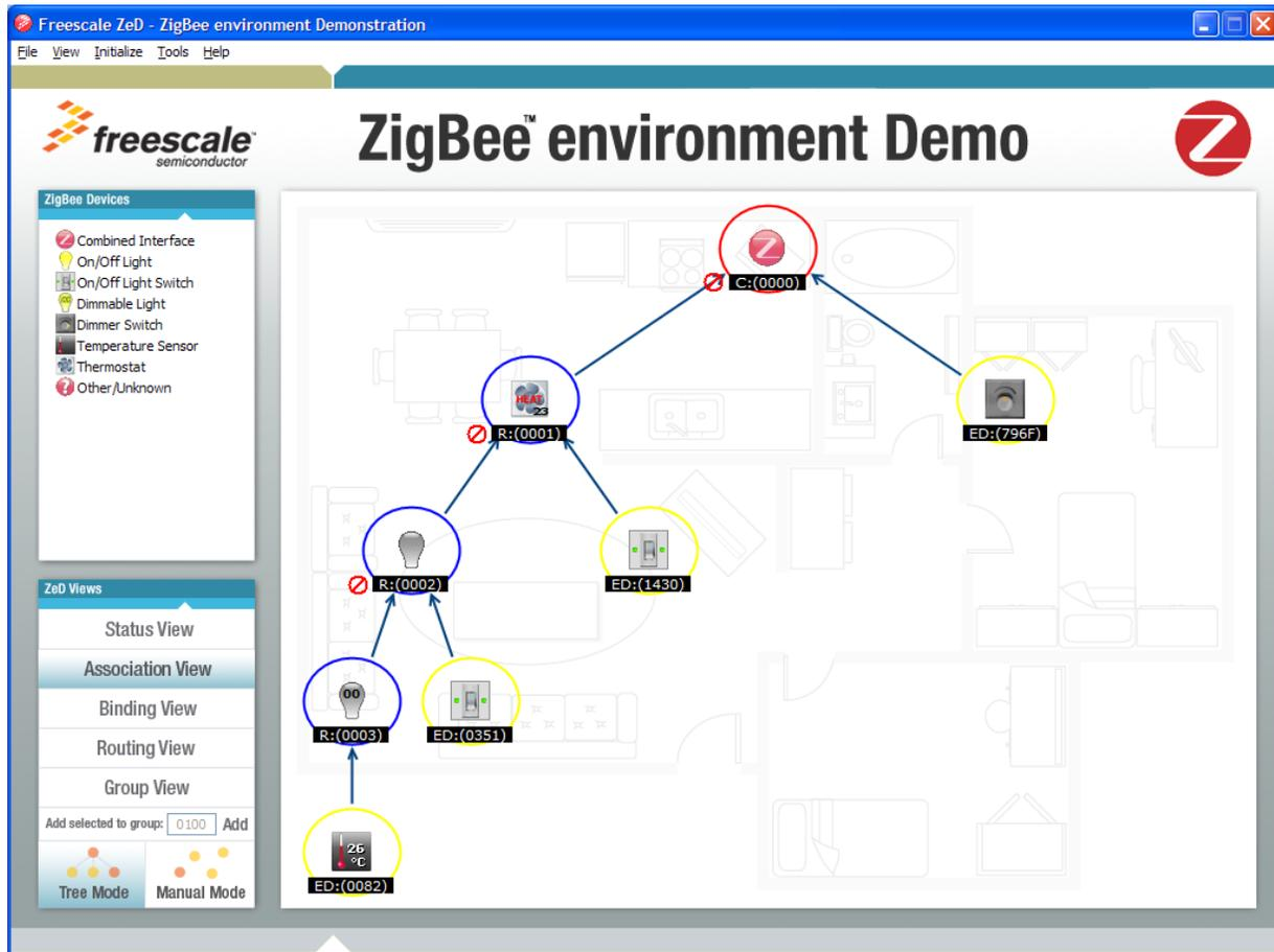
**Figure 5-8. High Depth Network**
