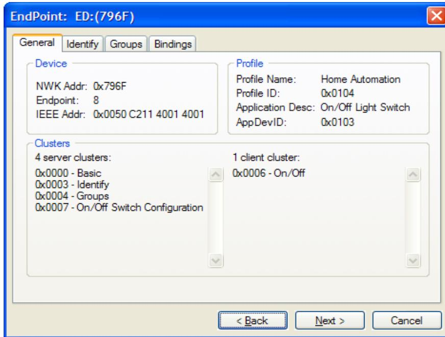
**Figure 4-10. Endpoint Properties Window**
