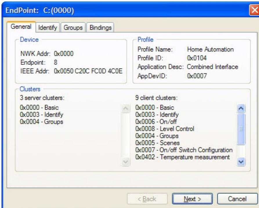
**Figure 7-1. General Tab of the Endpoint Properties Window**
