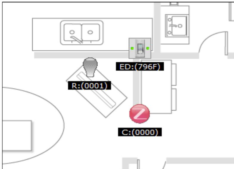
Figure 4-3. ZeD Main Window Showing On/Off Light Icon (Bulb Off State)
