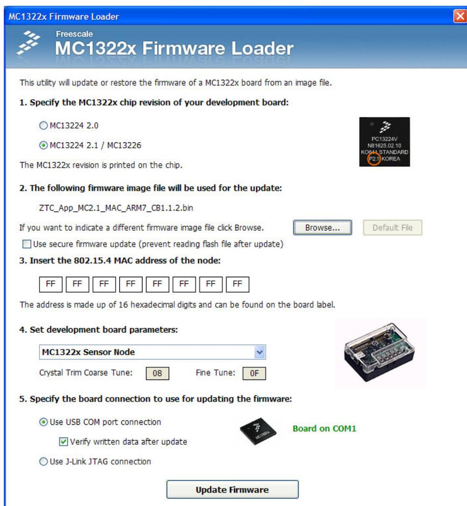
**Figure 2. Test Tool MC1322x Firmware Loader**
