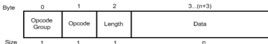
**Figure 4-1. Data Format (Upper Host and Lower Embedded Software)**
