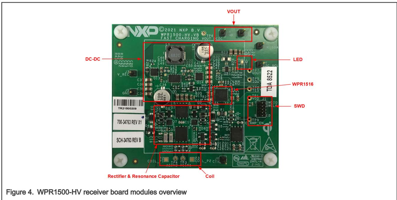
Figure 4. WPR1500-HV receiver board modules overview
