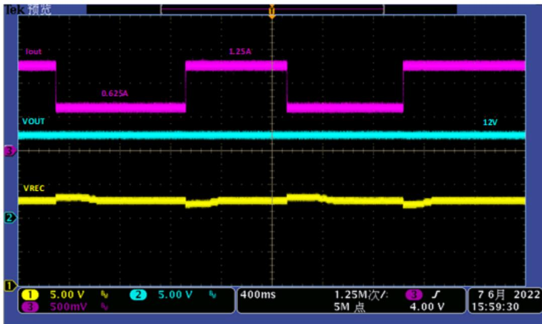
Figure 20. WPR1500-HV board load Step/Dump wave
