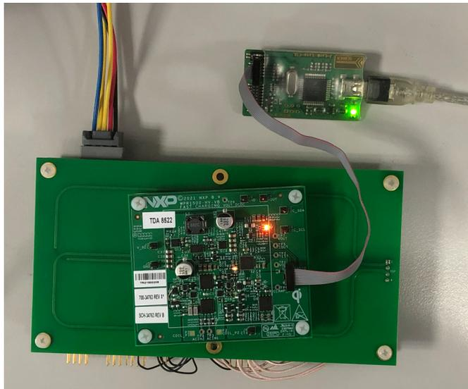
Figure 6. Monitoring by FreeMASTER connections
