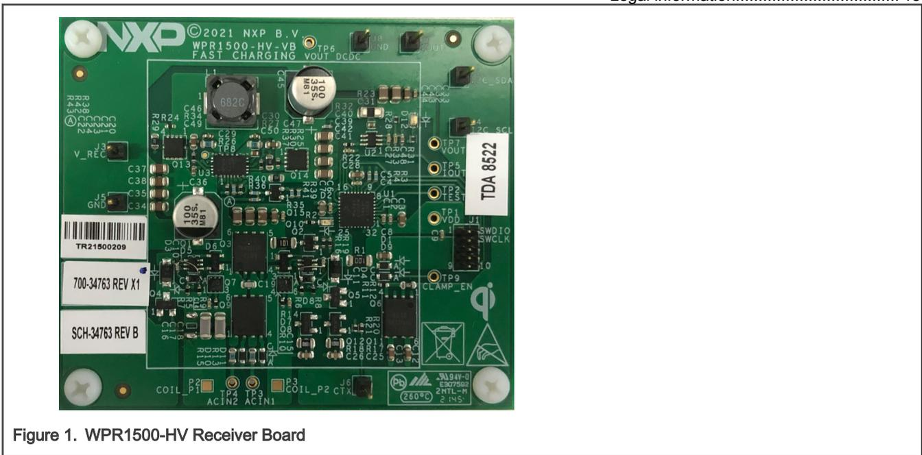
Figure 1. WPR1500-HV Receiver Board
