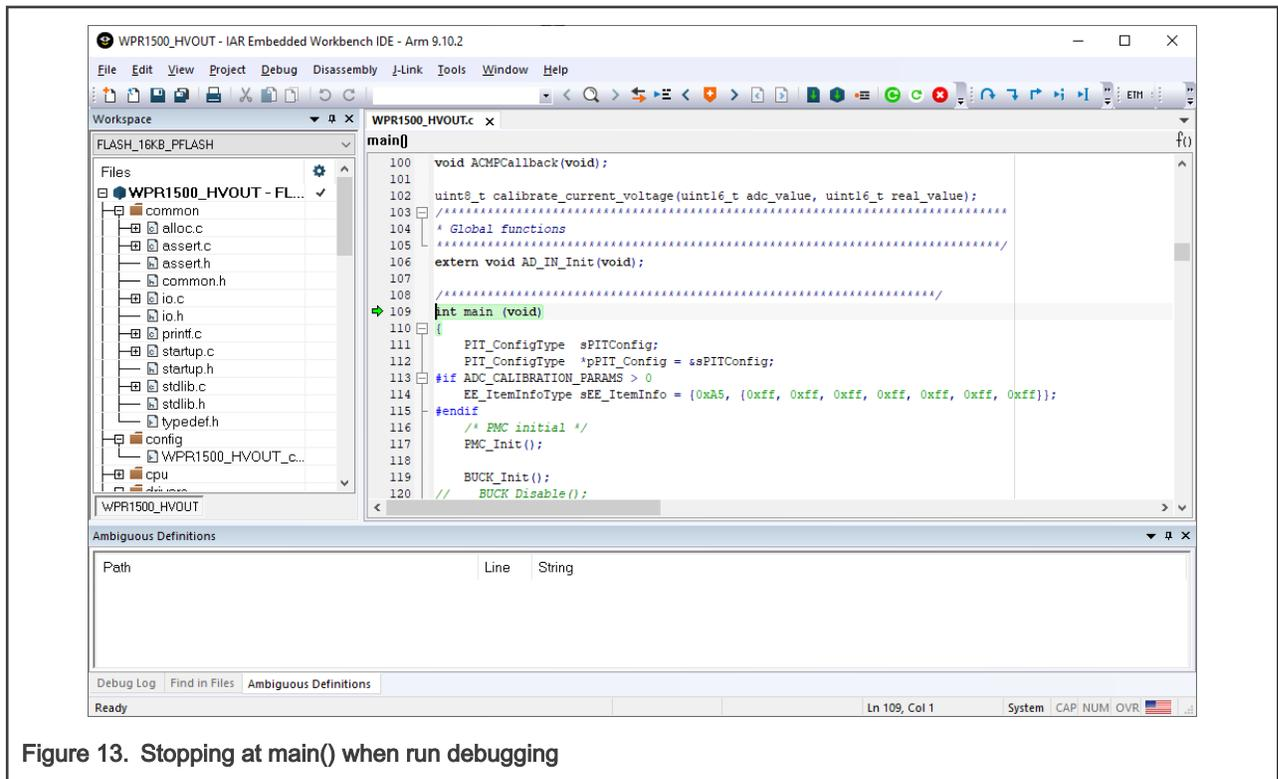
Figure 13. Stopping at main() when run debugging
