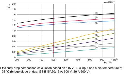
(1) One diode bridge (eff\_drop\_Diode\_125deg\_onePoVin\_rms)
