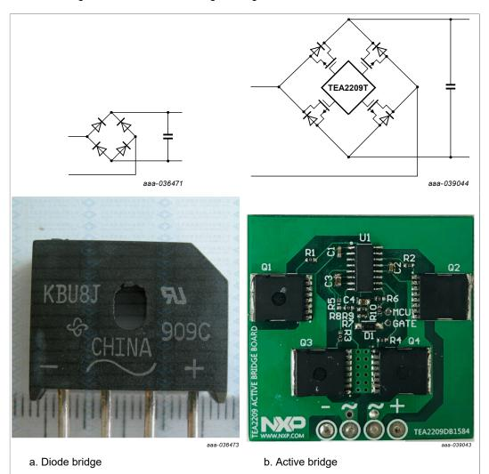
Figure 4. Diode bridge configuration versus TEA2209DB1584 demo board typical configuration
