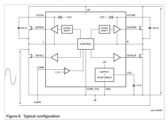
The control circuit of the TEA2209T senses the polarity of the mains voltage between pins L and R. Depending on the polarity, either GATELL or GATELR is switched on. The comparator in the control circuit, which compares the L and R voltages, has thresholds of 250 mV and -250 mV depending on the slope polarity. If the difference voltage between L and R is less than 250 mV both GATELL and GATELR are low.
