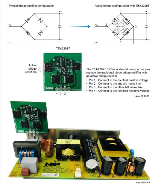
Figure 8. TEA2209T test setup on TEA2016DB1519
