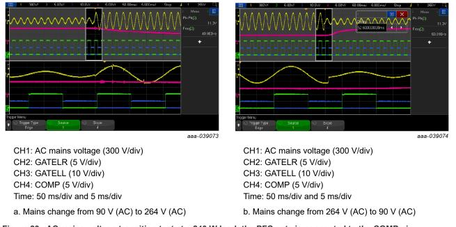
Figure 23. AC mains voltage transition test at a 240 W load; the PFC gate is connected to the COMP pin
