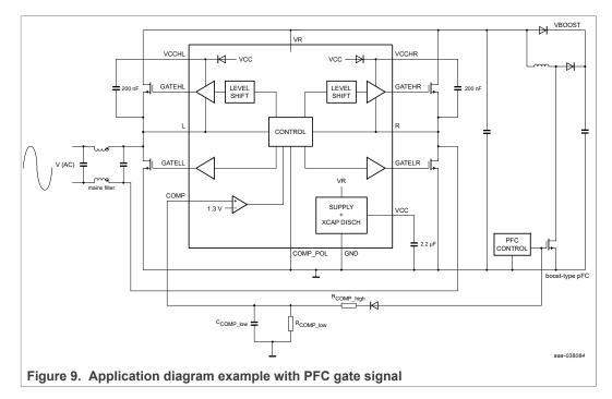
The TEA2209DB1584 implements an external RC filter with  $R_{COMP\_high} = 18 k\Omega$ ,  $R_{COMP\_low} = 180 k\Omega$ ,  $C_{COMP\_high} = 2.2 \,\mu\text{F}$  and 1N4148. To adjust the output power level which disables gate drivers, change  $R_{COMP\_high}$ . As reducing  $R_{COMP\_high}$  value, gate drivers can be disabled at lower power levels. Section 6.8.2 gives the test result with the TEA2016DB1519.
