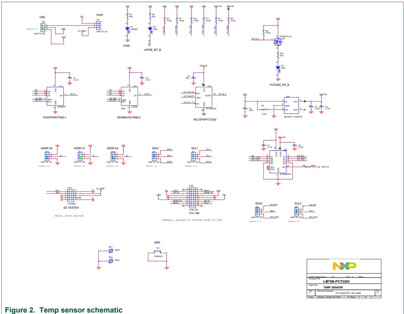
Figure 2. Temp sensor schematic
