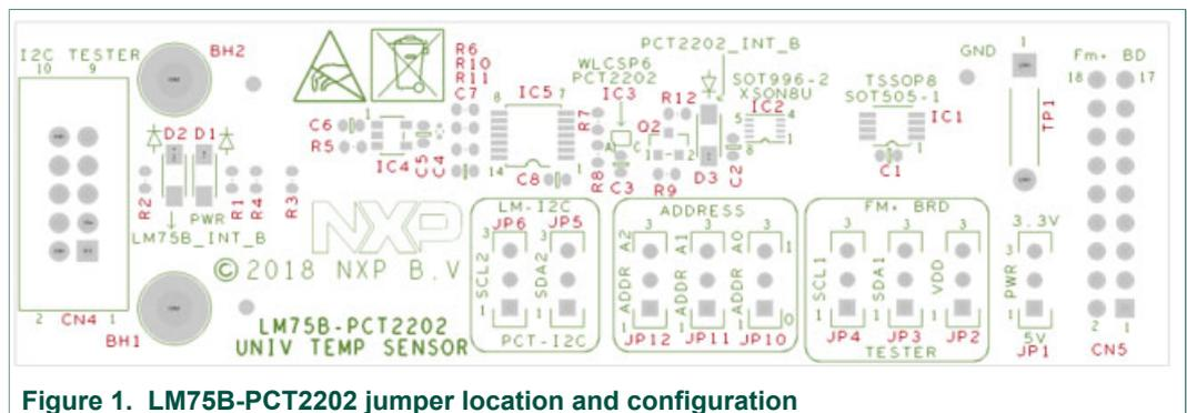
Figure 1. LM75B-PCT2202 jumper location and configuration
