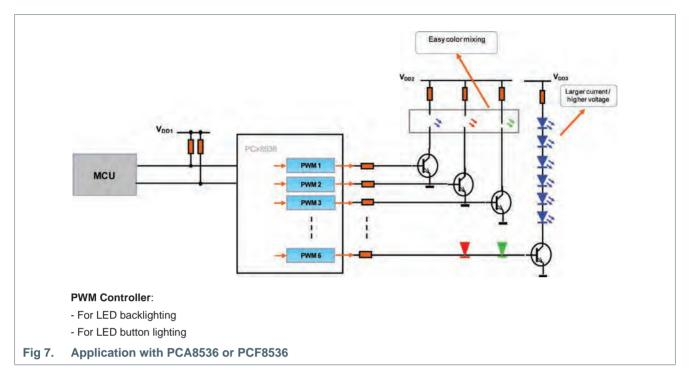
The LCD frame frequency and the PWM frequency are derived from the same clock source and can be programmed independently; it will be enough to program the two frequencies more than 50 Hz apart to prevent any display flickering across the operating temperature range and production spread.
