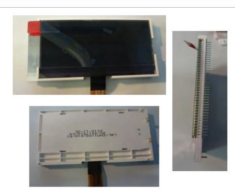
Fig 5. LCD with backlight LEDs in a plastic frame
