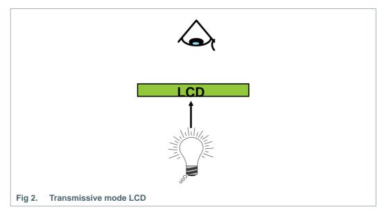
The reflective LCDs work best in an outdoor or well-lit environment; transmissive LCDs work best in low-light conditions, with the backlight continuously on. Transmissive LCDs guarantee much better optical performance but require a backlight, a circuitry to drive the backlight, and this implies higher power consumption.
