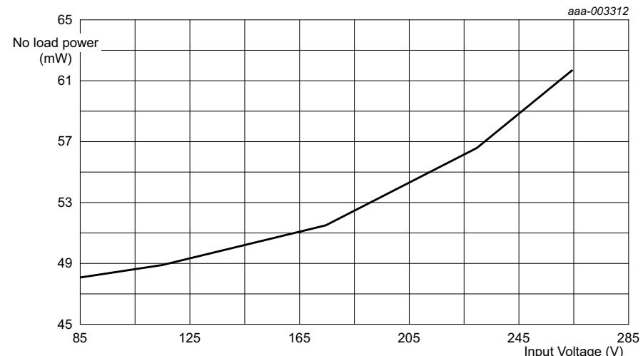
**Fig 3. No-load input power consumption**
