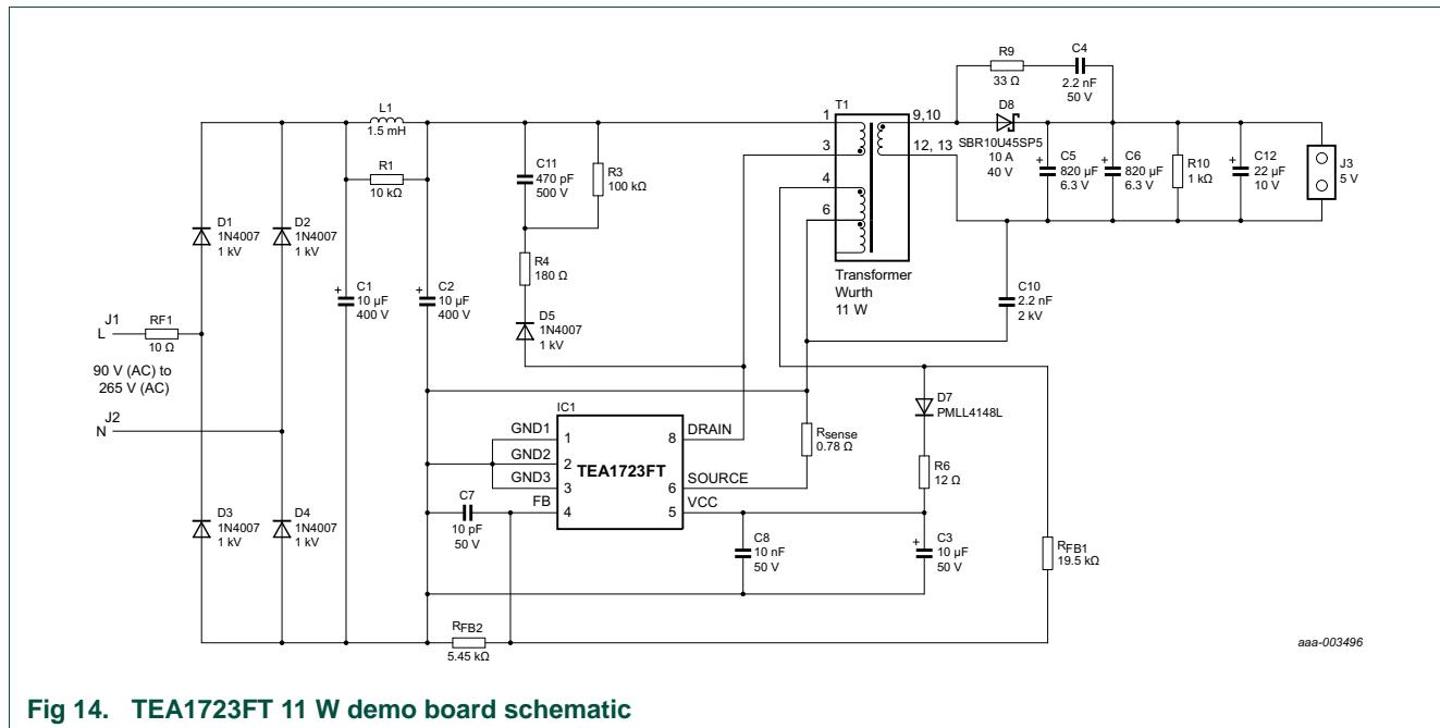
Fig 14. TEA1723FT 11 W demo board schematic
