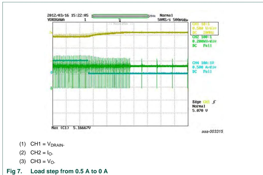
**Fig 7. Load step from 0.5 A to 0 A**
