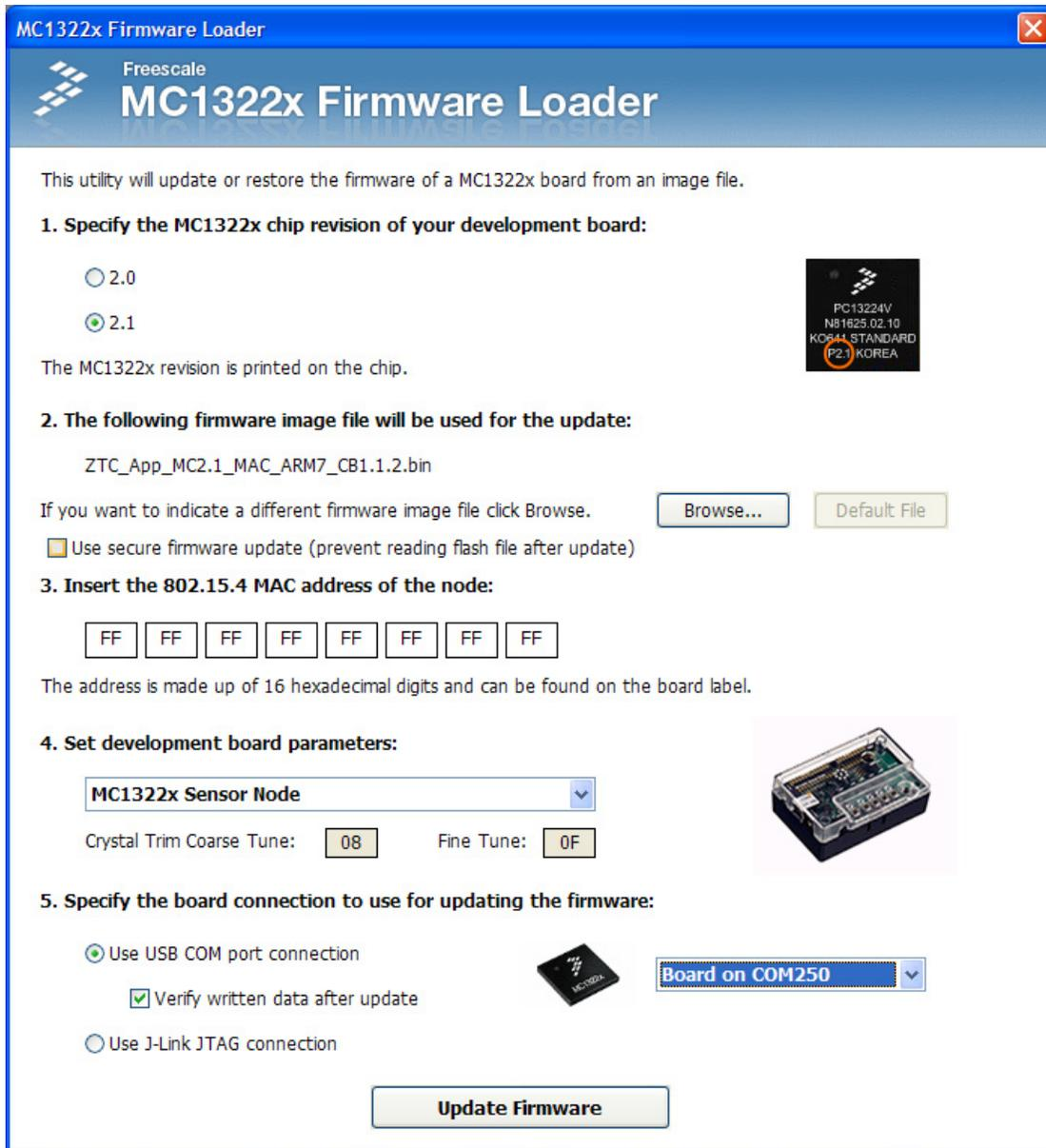
Figure 4-3. MC1322x Firmware Loader Main Window
