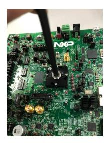
2. Remove the socket cover by turning it to the left and lifting up. Set it aside.
