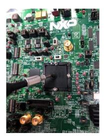
4. Using the vacuum tool, pick up the S32G device and place it in the socket base. Make sure that the polarity mark matches the socket polarity mark indicated by the dots.
