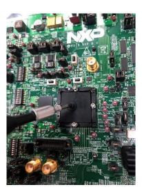
7. Replace the socket cover and turn to the right to lock in place.
