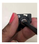
6. Using the vacuum tool, install the compression plate on top of the S32G device.
