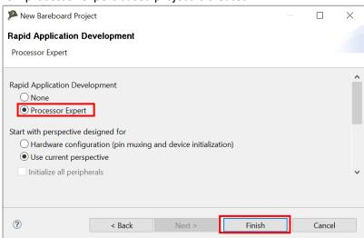
g. The Processor Expert view is opened automatically. Processor Expert provides a GUI interface to easily configure pins, clock, peripherals and middleware such as FreeMASTER. Start development by adding the desired components from **Components Library**.
