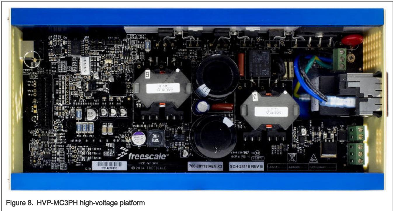
Figure 8. HVP-MC3PH high-voltage platform
