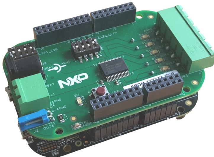
**Figure 1. Typical FRDM-17XSF5-EVB configuration**
