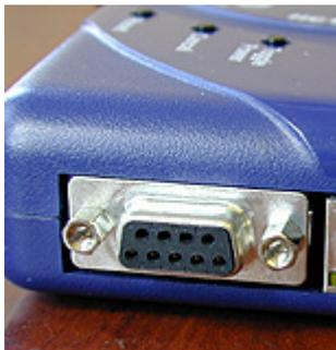
**Figure 3-3: Cyclone PRO RS232 Connector**
