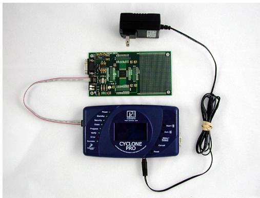
**Figure 3-18: Via Cyclone PRO Board Power and Pin 6 of Cyclone PRO BDM Connector**
