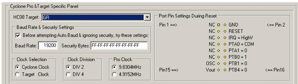
**Figure 13-9: 68HC908GR16/32 MON08 Pinout**
