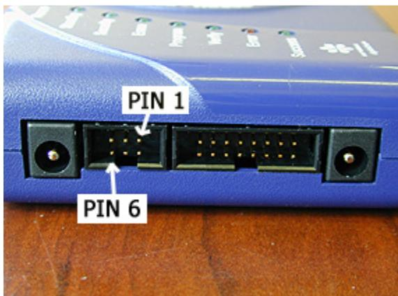
**Figure 3-7: 6 Pin BDM Connector Pin Connections**
