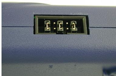
**Figure 3-21: Jumper Settings For Power IN Jack And MON08 Header Pin 15**
