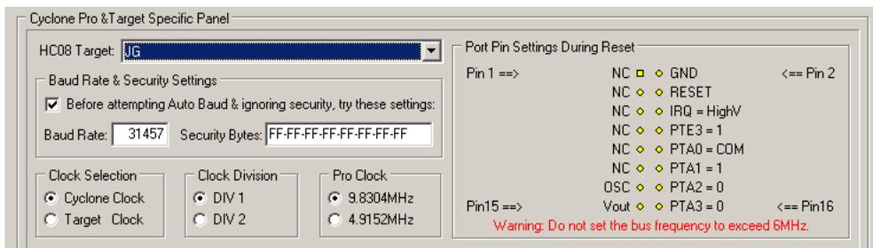
**Figure 13-16: 68HC908JG Family MON08 Pinout**
