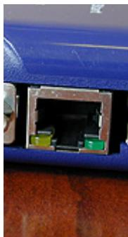
**Figure 3-4: Cyclone PRO Ethernet Connector**
