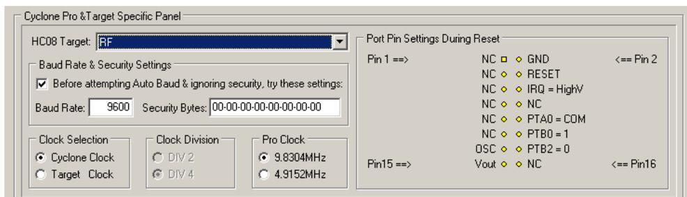
**Figure 13-35: 68HC908RF Family MON08 Pinout**
