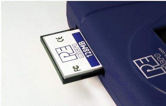
**Figure 3-22: CompactFlash Port**
