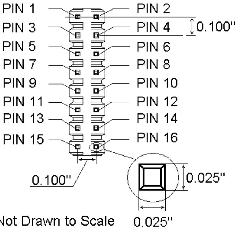
Figure 3-8: 16-Pin Header Mechanical Drawing
