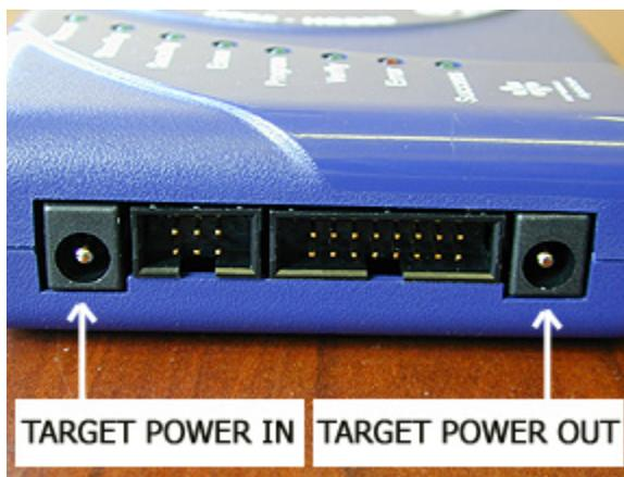
Figure 3-6: Power Connector Locations
