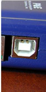
Figure 3-5: Cyclone PRO USB Connector
