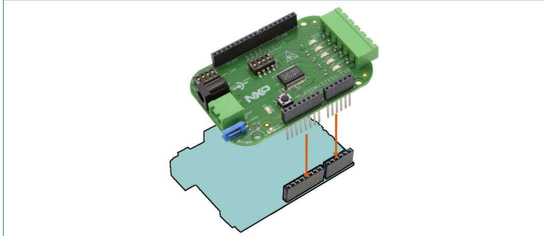
**Figure 10. Connecting the FRDM-32XSG-EVB to an Arduino board**
