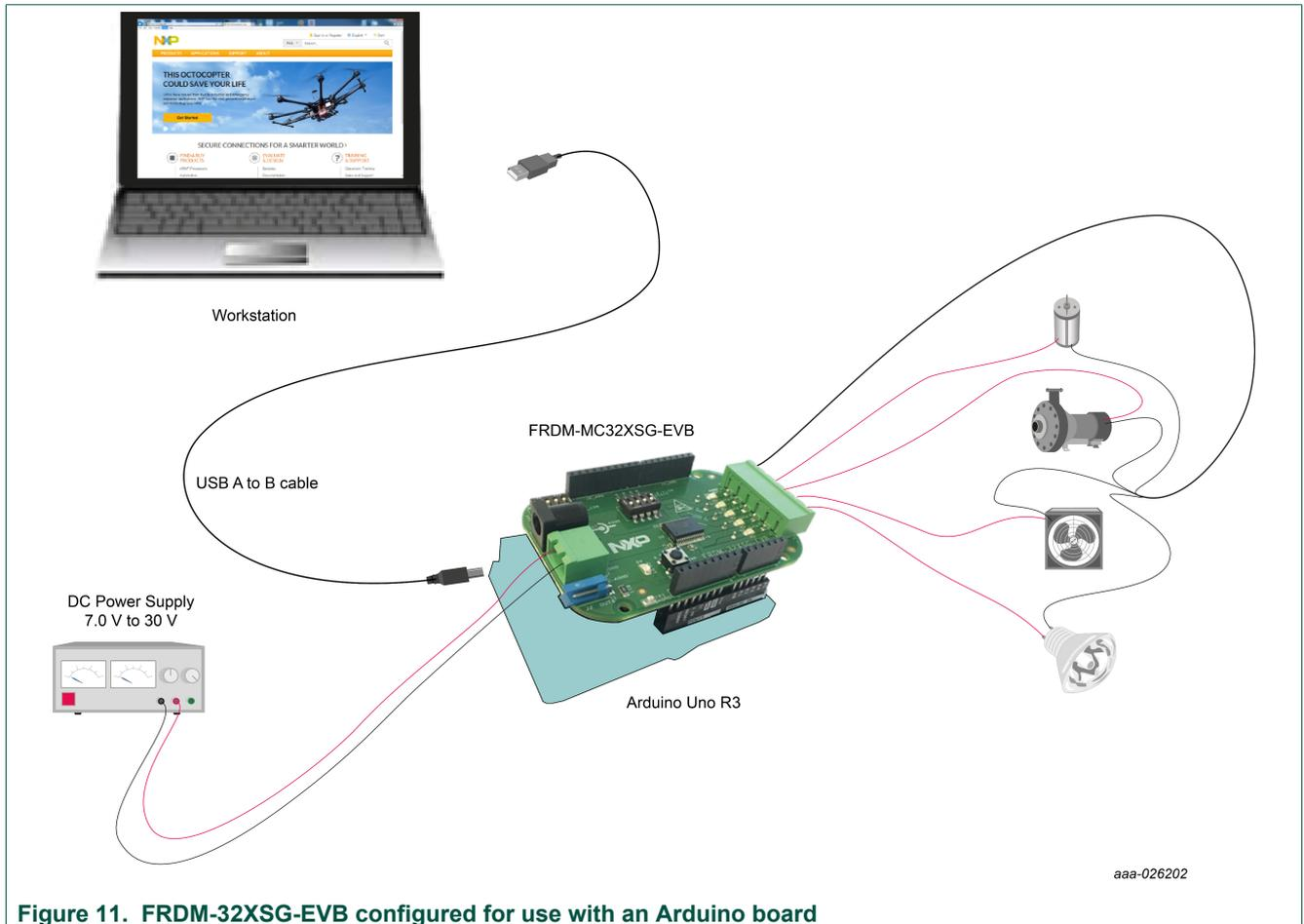
Figure 11. FRDM-32XSG-EVB configured for use with an Arduino board
