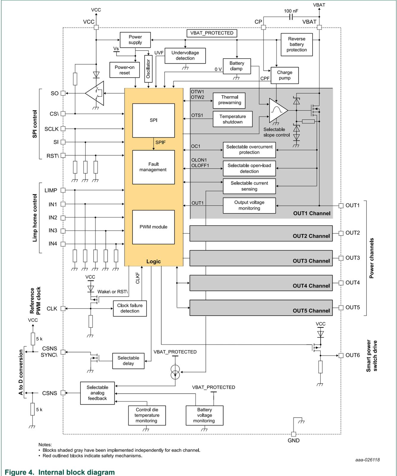
Figure 4. Internal block diagram
