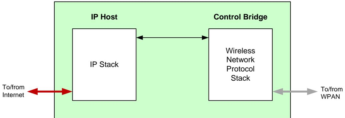
Figure 8: Basic Architecture of an IoT Gateway
