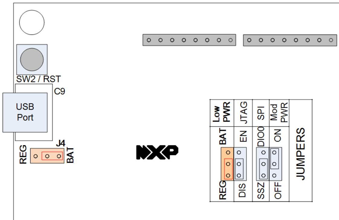
Figure 17: Locations of Power Selection Jumpers (J4 and Low PWR)
