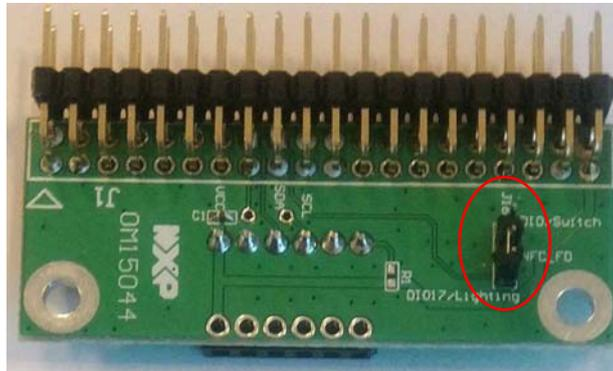
**Figure 33: J16 Jumper on OM15044 Adaptor**
