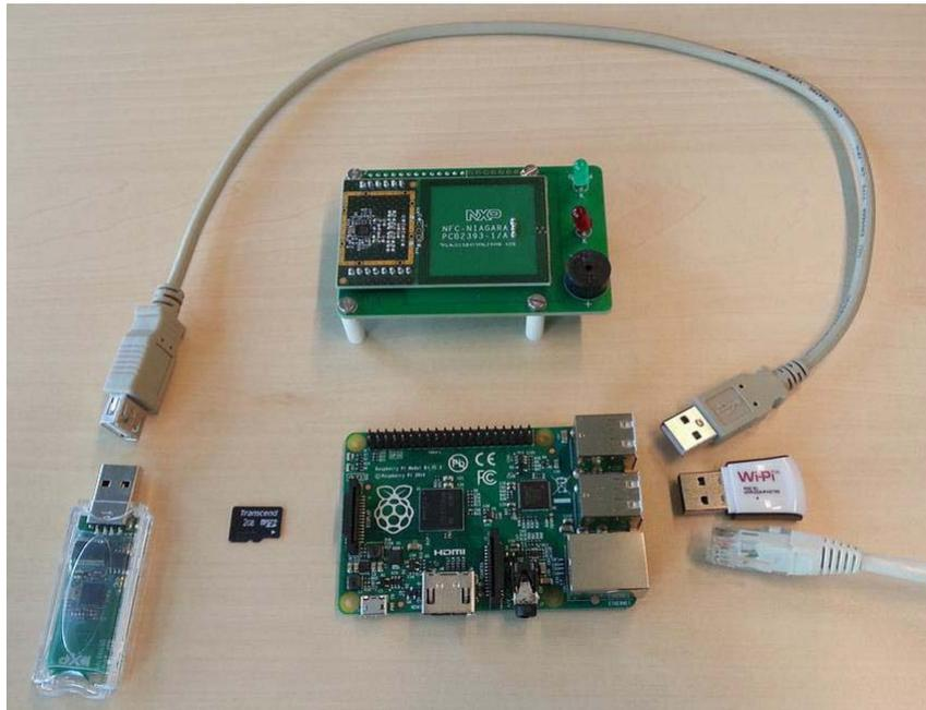
**Figure 29: Raspberry Pi Board and Accessories**
