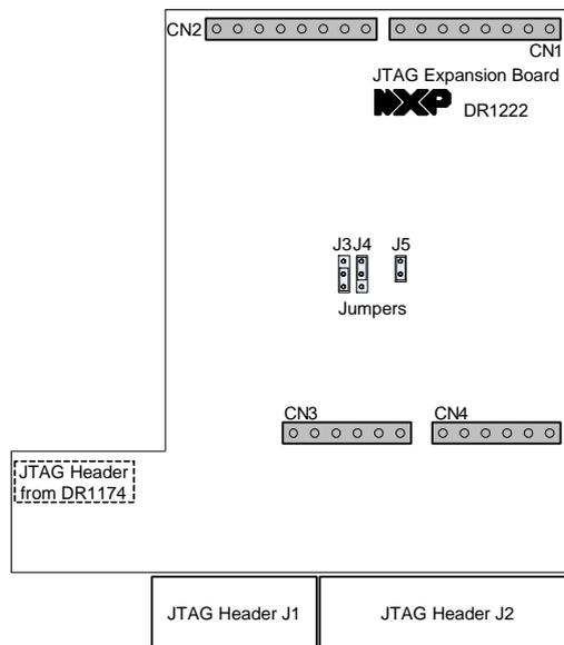
**Figure 26: JTAG Expansion Board Layout**
