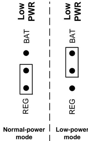
Figure 19: Lower-Power Mode Selection (using Low PWR Jumper)
