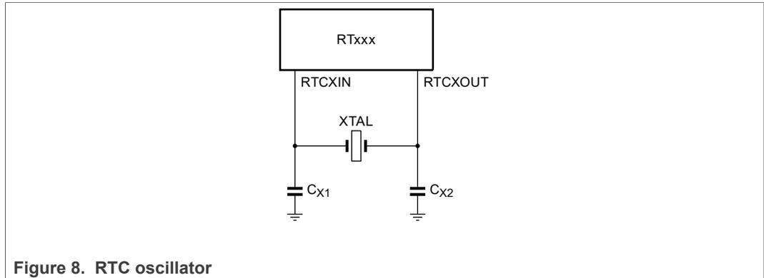
Figure 8. RTC oscillator
