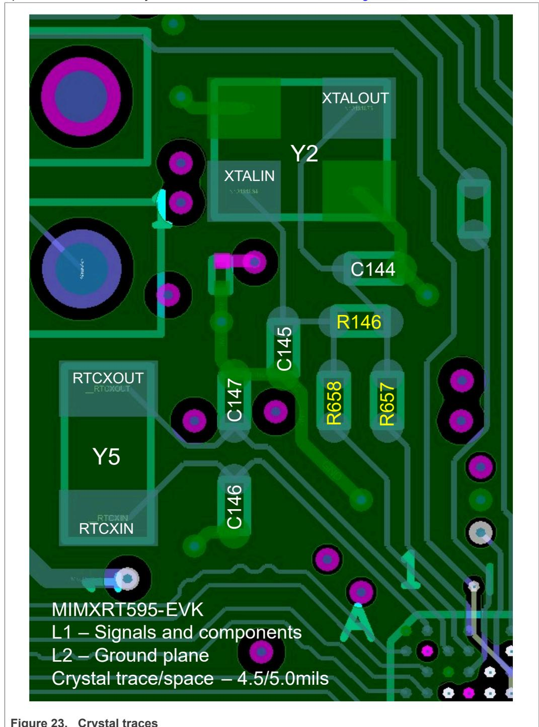
We recommend placing load capacitors for the RTC oscillator even when using internal capacitors, in case the internal capacitors do not have enough tuning resolution. It is important to maintain the RTC frequency accurately.
