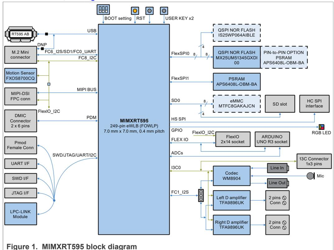
Figure 1. MIMXRT595 block diagram
