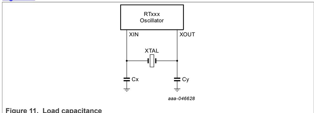
Figure 11. Load capacitance
