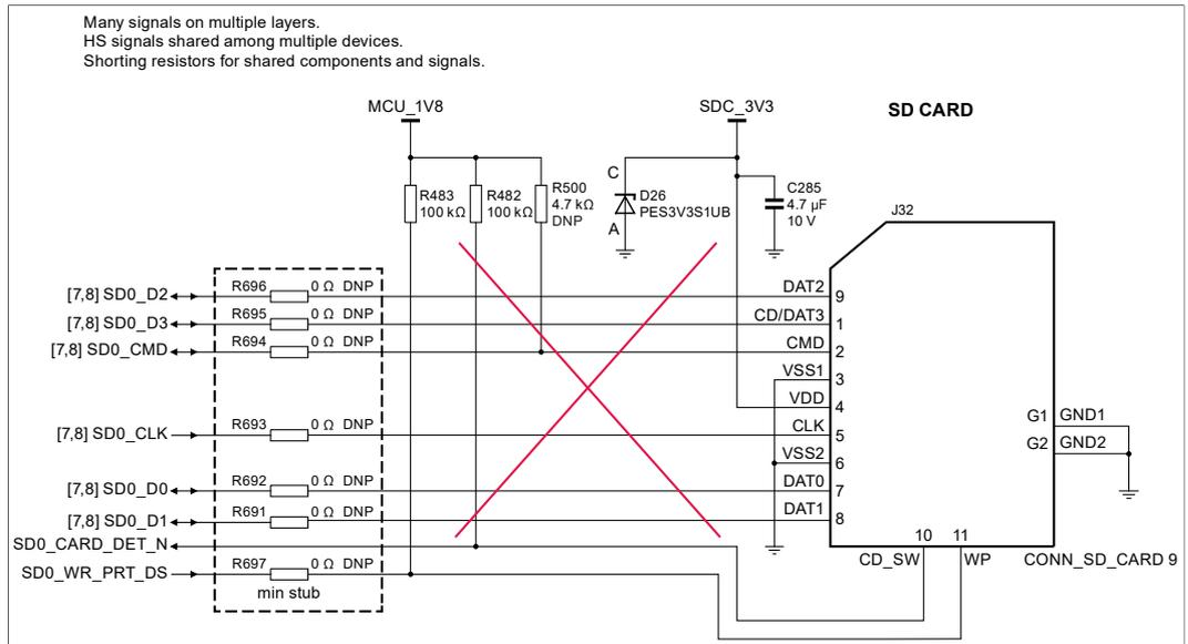
Figure 31. EVK SD card schematic
