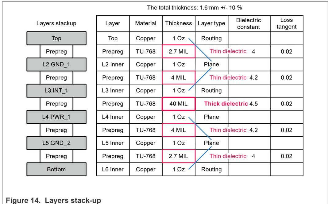
First, notice the dielectric thicknesses between the successive layers. L1 is tightly coupled to L2 with a 2.7 mil dielectric. L3 is tightly coupled to L2 with a 4 mil dielectric.
