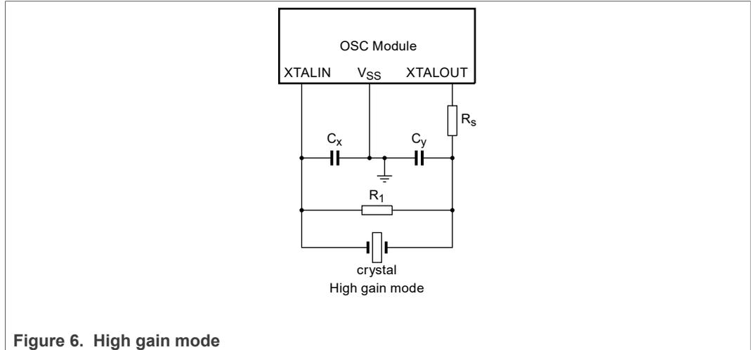
Figure 6. High gain mode
