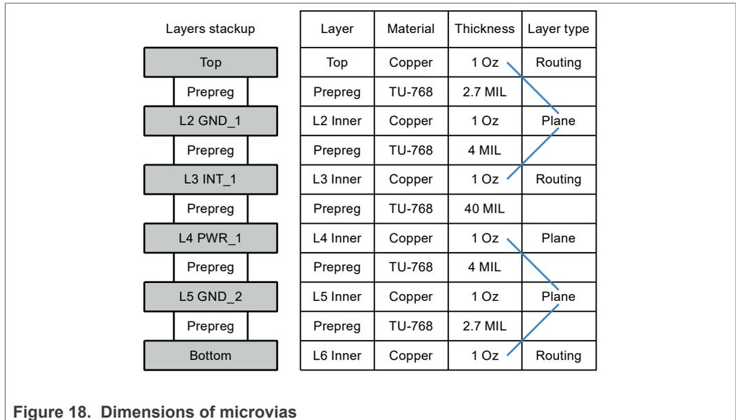
Figure 18. Dimensions of microvias
