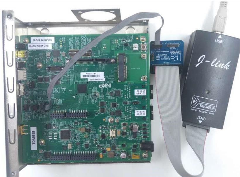
**Figure 1. Connecting Jlink to LS1012ARDB**
