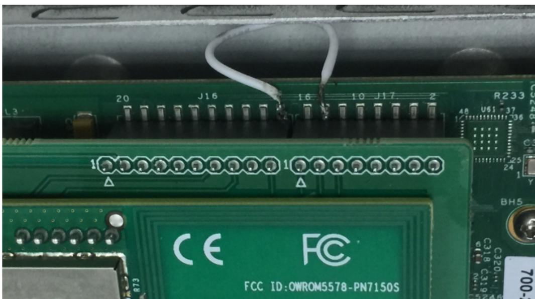
Figure 11. NFC hardware rework on LS1012ARDB board
