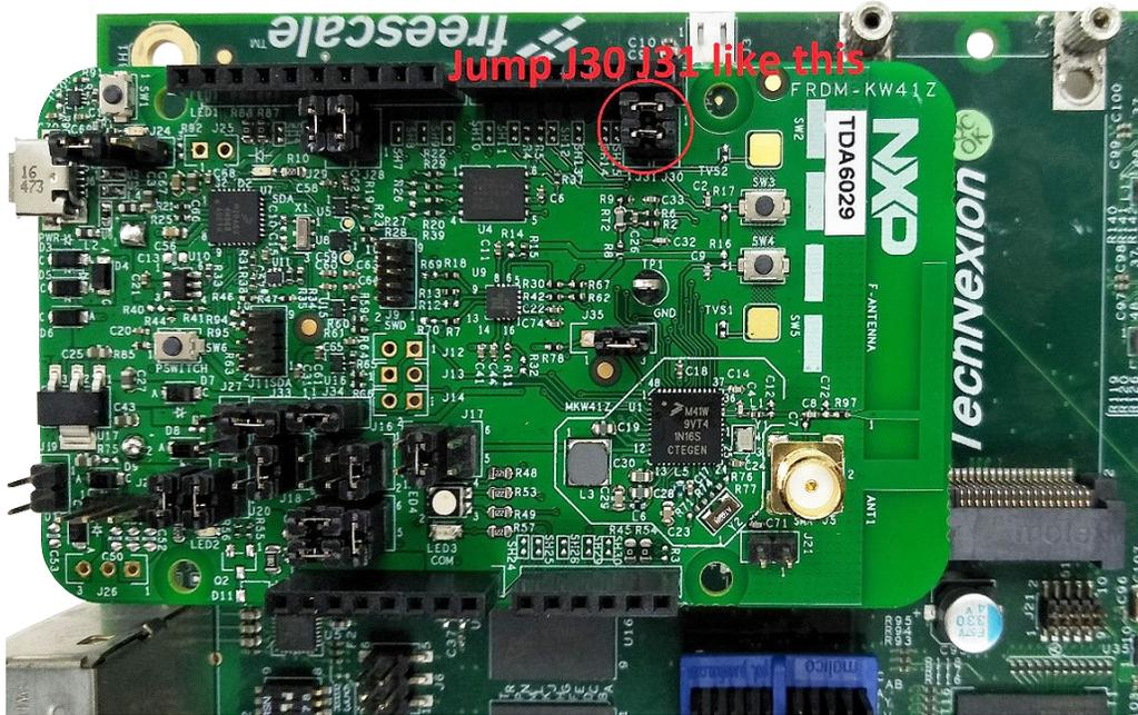
Figure 4. Jumper settings on FRDM-KW41Z board A
