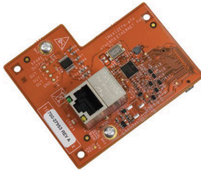
Figure 4. Atheros Ethernet add on card (IMXA12ETH-ATH)
