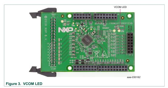
The VCOM LED indicates when the device is in normal mode. Upon reset, the MC33772B enters into normal mode (VCOM turns on). If there is no activity on the bus after a timeout period of 60 seconds, the device enters low-power idle mode (VCOM turns off). Once the device is initialized, if no communication occurs on the bus after one second, the device resets and the LED turns off (VCOM off). Depending on the device settings, the VCOM LED may flash 0.1...8 seconds during cyclic acquisition.
