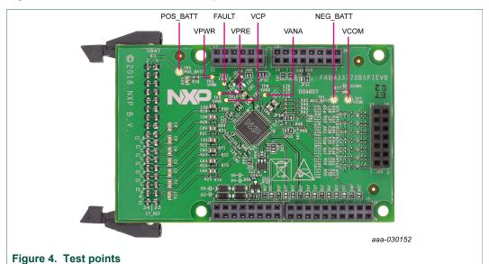
The following test points provide access to various signals to and from the board.
