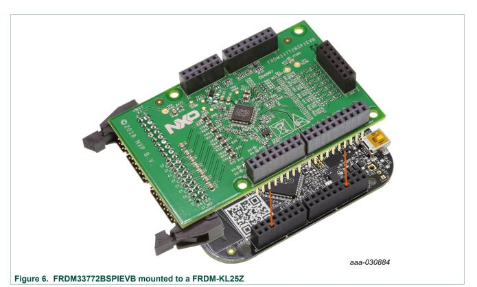
The board must be modified to be compatible with each specific Freedom board. This modification is described in <u>Section 5.1 "Compatible NXP MCU development platforms"</u>.
