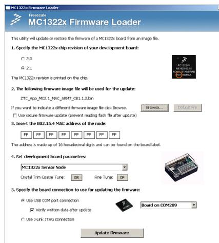
**Figure 4-10. MC1322x Firmware Loader Window**
