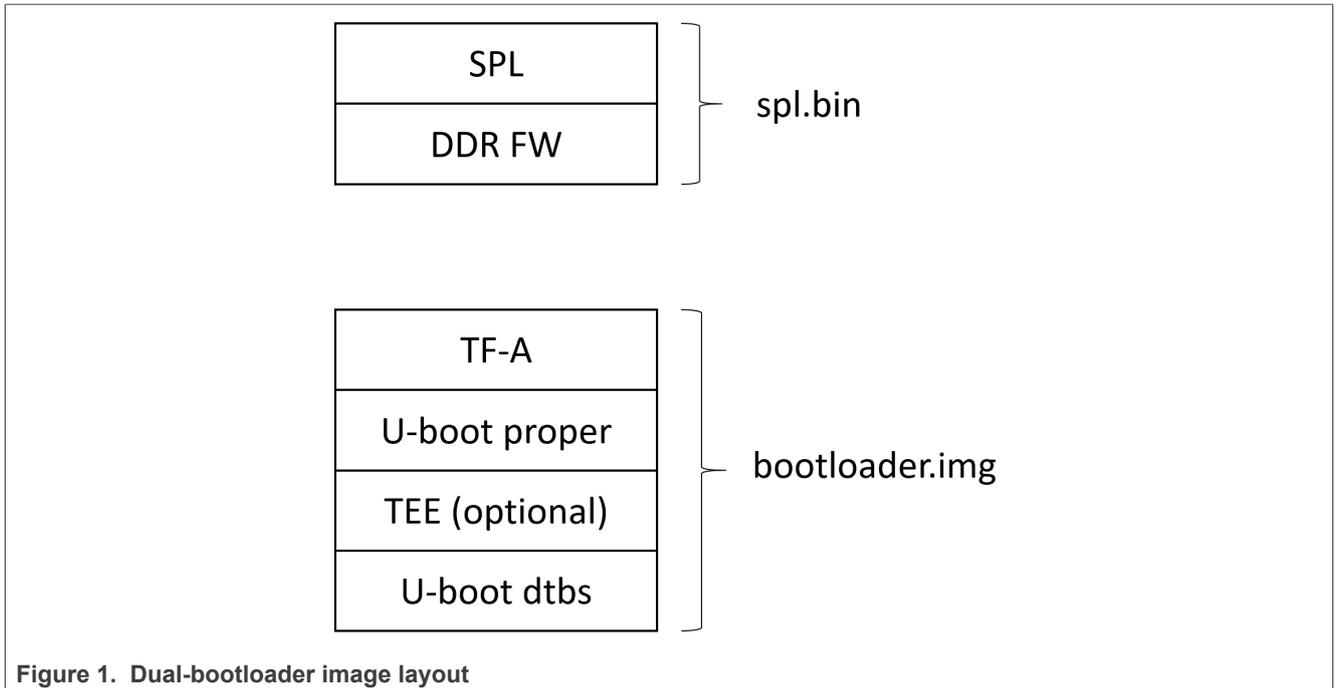
Figure 1. Dual-bootloader image layout
