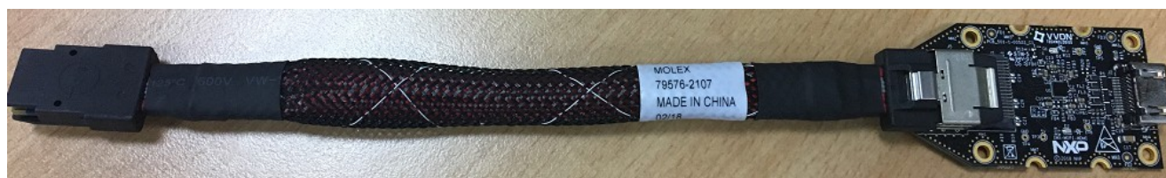
Figure 7. i.MX mini SAS cable with DSI-to-HDMI adapter
