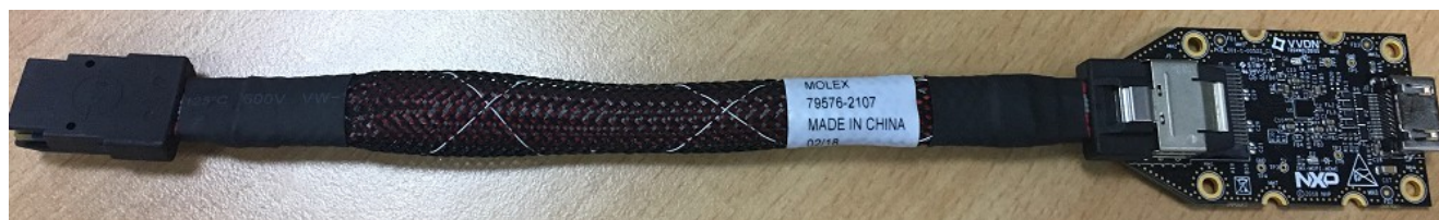
Figure 2. i.MX mini SAS cable with DSI-to-HDMI adapter
