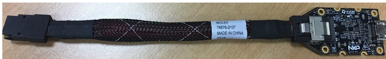
Figure 9. i.MX mini SAS cable with DSI-to-HDMI adapter
