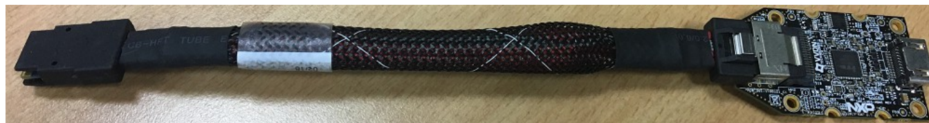
Figure 15. i.MX mini SAS cable with LVDS-to-HDMI adapter
