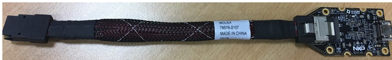
Figure 14. i.MX mini SAS cable with DSI-to-HDMI adapter
