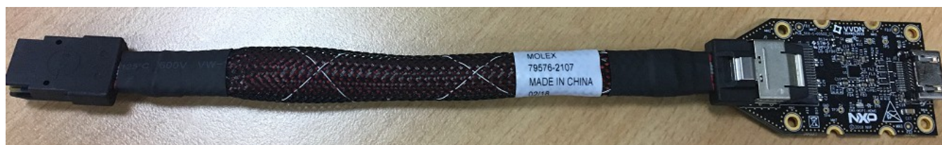
Figure 20. i.MX mini SAS cable with DSI-to-HDMI adapter
