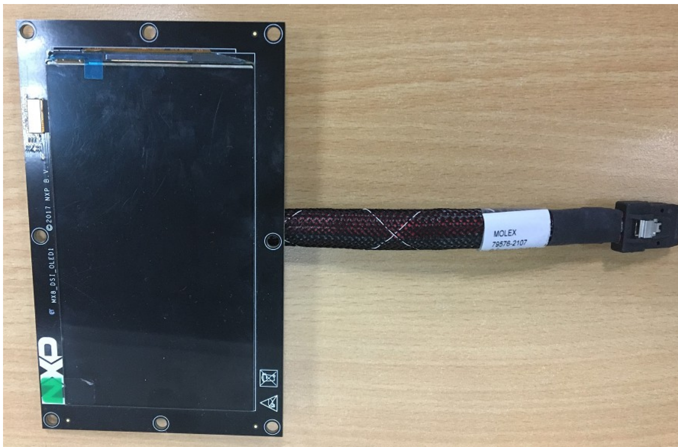
Figure 4. i.MX MIPI panel
