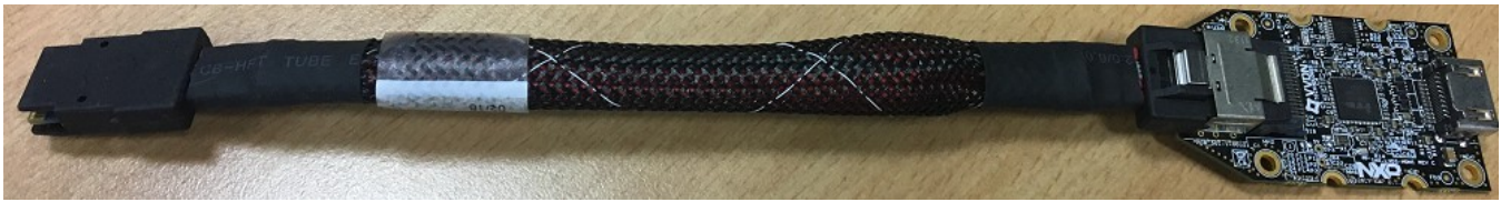
Figure 9. i.MX mini SAS cable with LVDS-to-HDMI adapter
