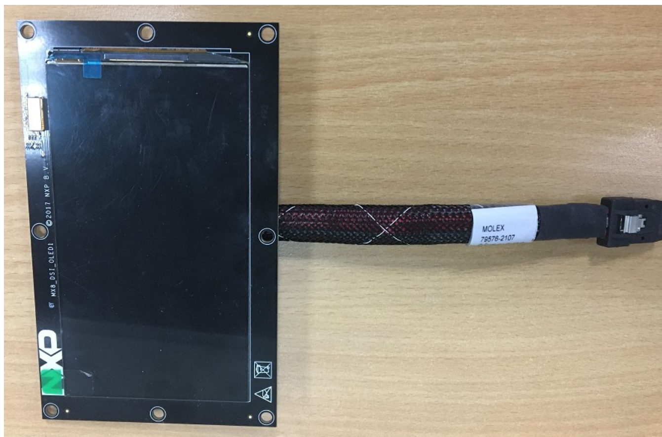
Figure 14. i.MX MIPI panel
