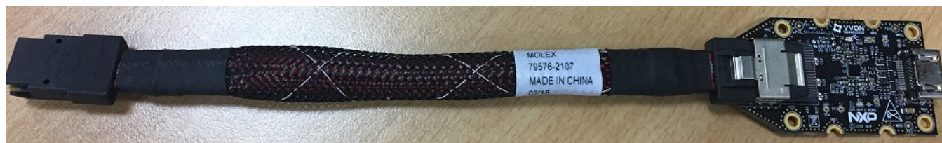
Figure 8. i.MX mini SAS cable with DSI-to-HDMI adapter
