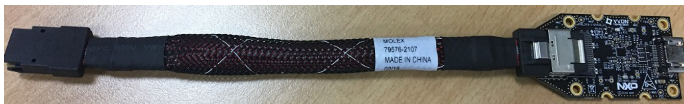
Figure 13. i.MX mini SAS cable with DSI-to-HDMI adapter
