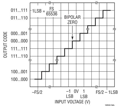
Figure 4b. Bipolar Transfer Characteristics (UNI = 0)
