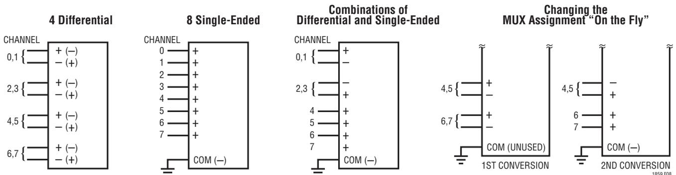
Figure 8. Examples of Multiplexer Options on the LTC1857/LTC1858/LTC1859
