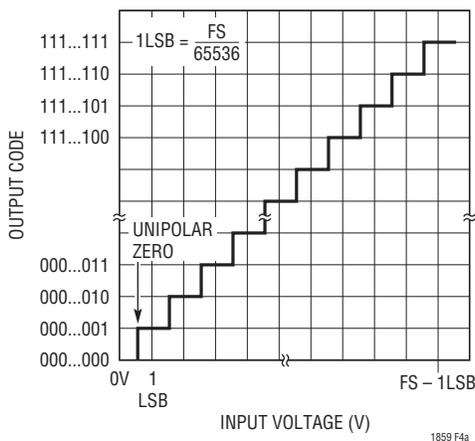
Figure 4a. Unipolar Transfer Characteristics (UNI = 1)
