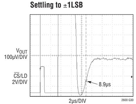
$V_{CC} = 5V, V_{REF} = 4.096V$
