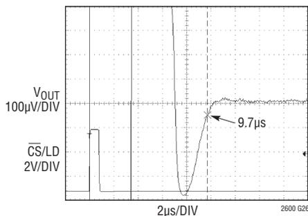
$V_{CC} = 5V$ ,  $V_{REF} = 4.096V$
