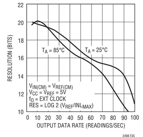
**Figure 35. Resolution ( $INL_{\text{MAX}} \leq 1\text{LSB}$ ) vs Output Data Rate and Temperature**
