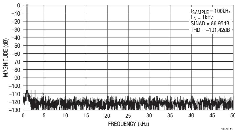
Figure 12. LTC1859 Nonaveraged 4096 Point FFT Plot
