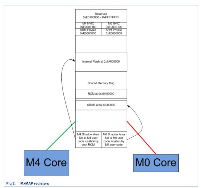
Q: How can the M0 and the M4 execute different code at the same address?
