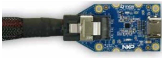
Figure 161. MIPI-DSI to HDMI interface
