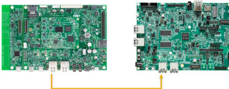
Figure 112. servo_motor example on i.MX RT1180 EVK as EtherCAT Slave
