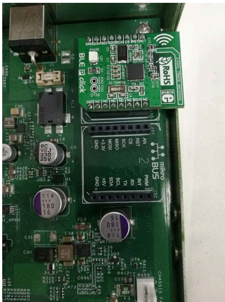
Figure 165. BLE P Click board hardware setup
