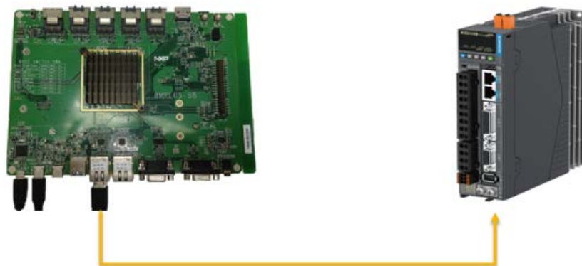
Figure 101. Running SOEM Servo Motor example on i.MX 8M Plus EVK (Inovance SV680 as EtherCAT Slave)
