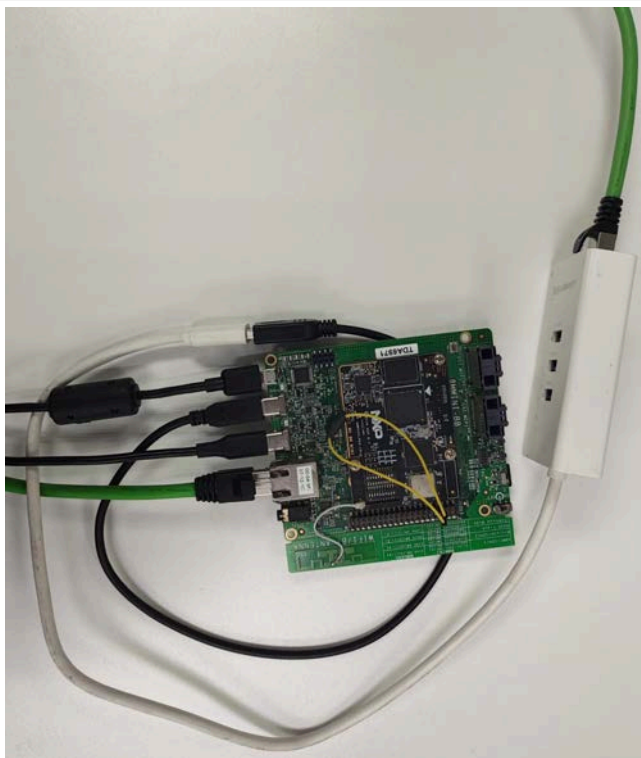
Figure 113. i.MX 8M Mini board connection
