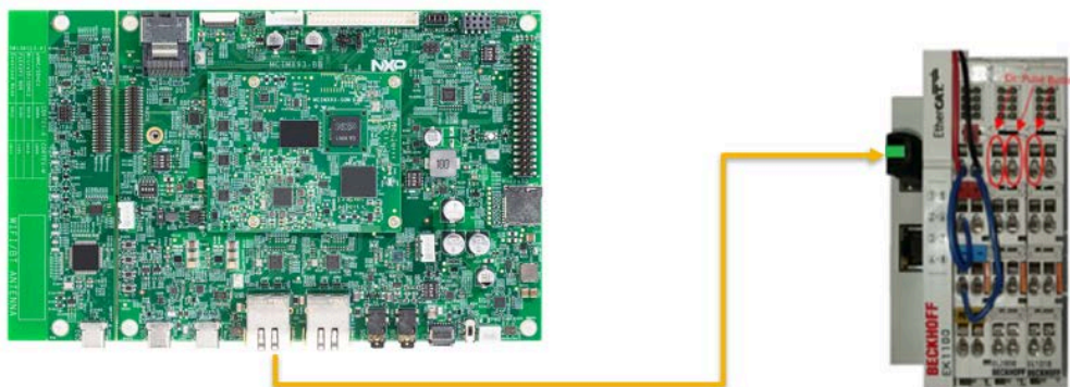
Figure 110. digital_io example for i.MX 93-EVK board
