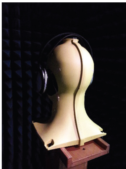
Figure 8. Radiated measurements of the antenna inside a headphone on a SAM phantom head mounted in an anechoic room
