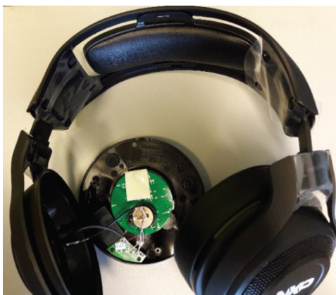
Figure 7. The conductive plane antenna integrated in a commercially available headphone
