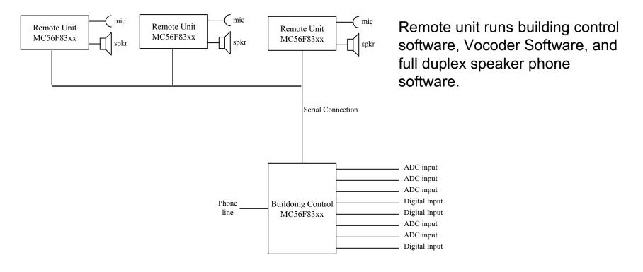
Control unit runs building control system, Vocoder Software, and full duplex speakerphone software.
