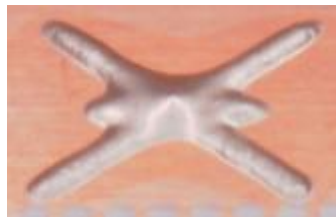
Dispense Patterns Visible solvent bleed out
