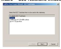
g. Select the appropriate predefined GCC toolchain or "Custom" to manually enter the location of a toolchain
