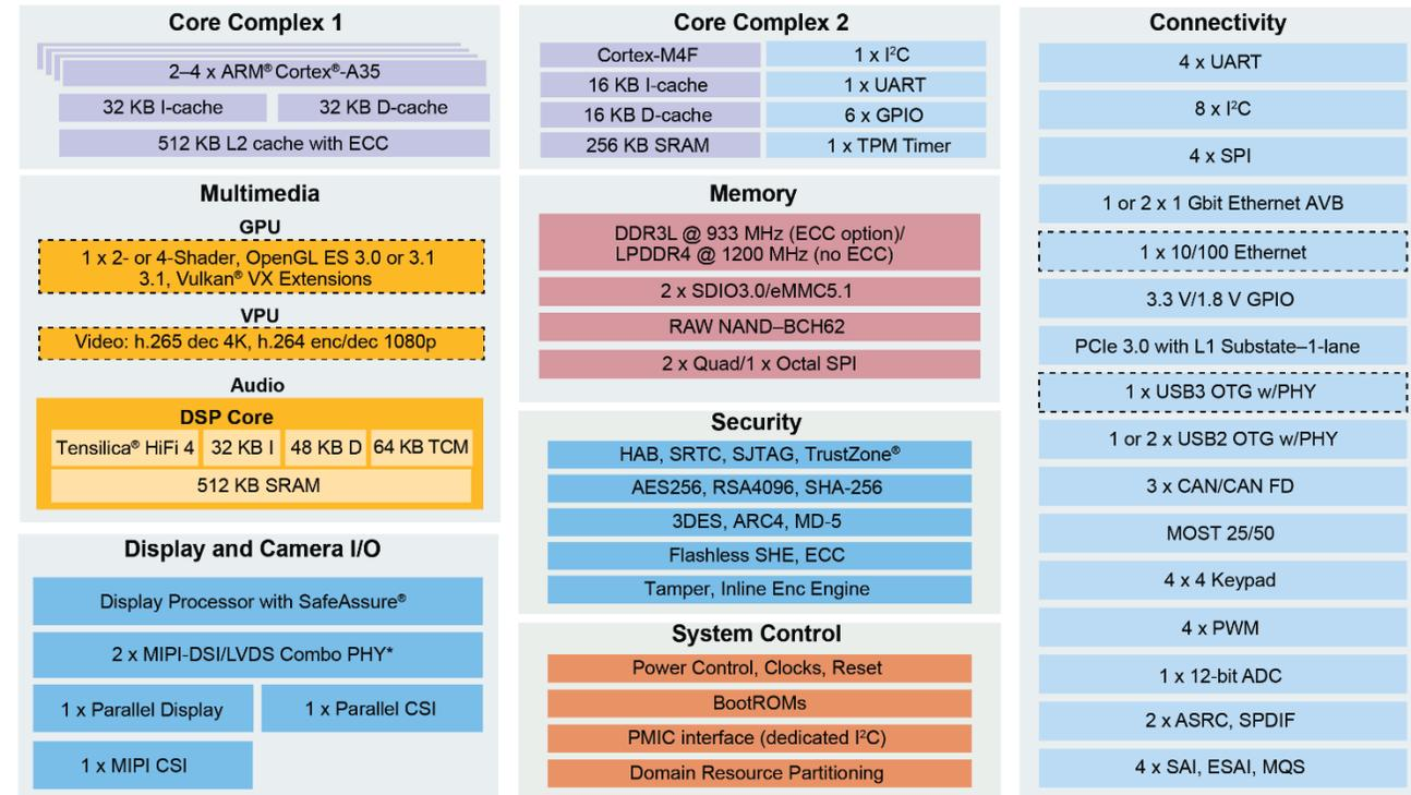
\* Each single PHY can either be a 1×4 lane MIPI-DSI or a 1×1 channel LVDS interface for a total of 2 display interfaces. In combination, the two PHYs can be configured to be a single 2-channel LVDS interface.
