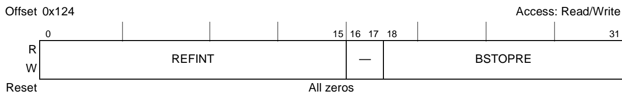
Figure 9-14. DDR SDRAM Interval Configuration Register (DDR_SDRAM_INTERVAL)
