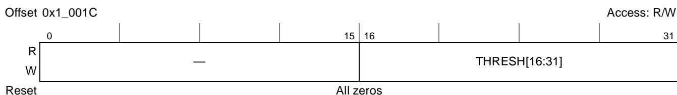
Figure 17-7. Performance Monitor Threshold Format
