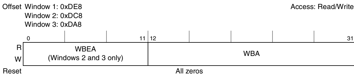
Figure 18-21. PCI Express Inbound Window Base Address Registers (PEXIWBAR n )
