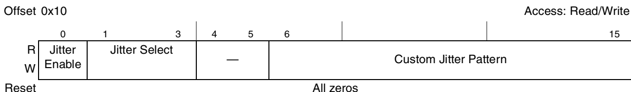
Figure 14-118. Jitter Diagnostics Register Definition
