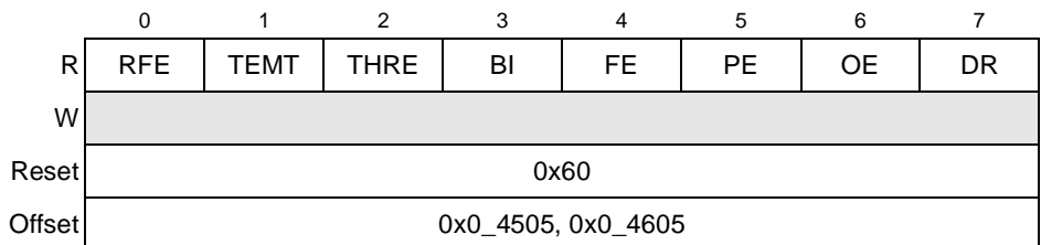
Figure 12-11. Line Status Register (ULSR)
