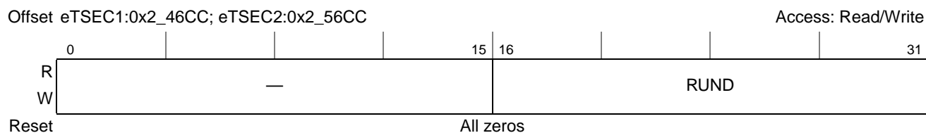
Figure 16-70. Receive Undersize Packet Counter Register Definition
