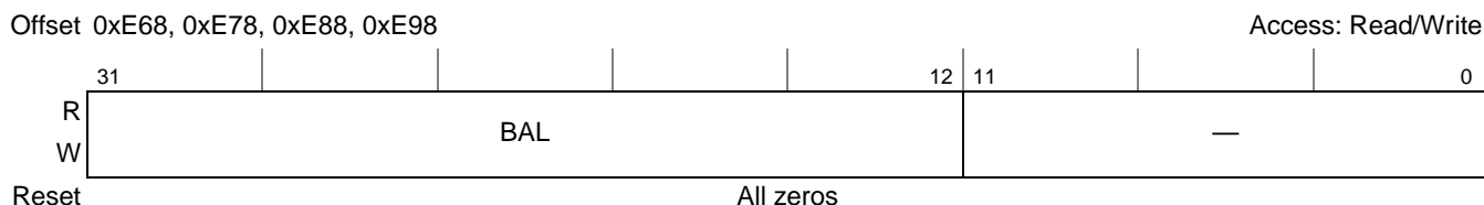
Figure 14-135. PCI Express RC Inbound Window Base Address Register Low n (PEX_RCIWBARL0–PEX_RCIWBARL3)
