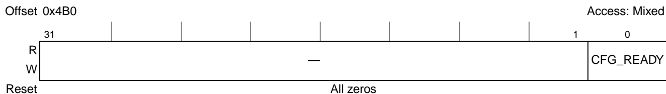
Figure 14-88. PCI Express Configuration Ready Register (PEX_CFG_READY)
