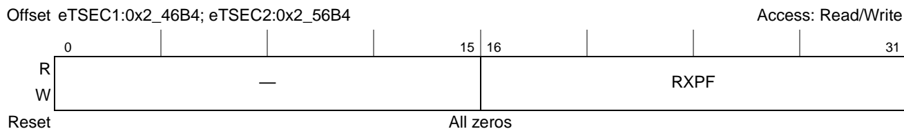
Figure 16-64. Receive Pause Frame Packet Counter Register Definition
