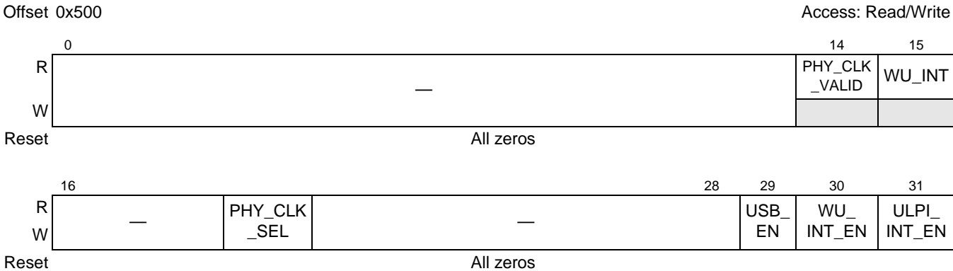
Figure 13-34. USB General-Purpose Register (CONTROL)
