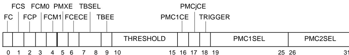
**Figure 11-1. Monitor Mode Control Register 0 (MMCR0)**
