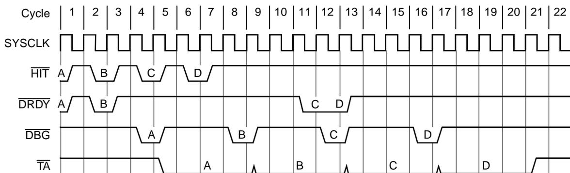
Cycles 1, 3, 5, and 7: The device asserts  $\overline{\text{HIT}}$  for transactions A, B, C, and D.
