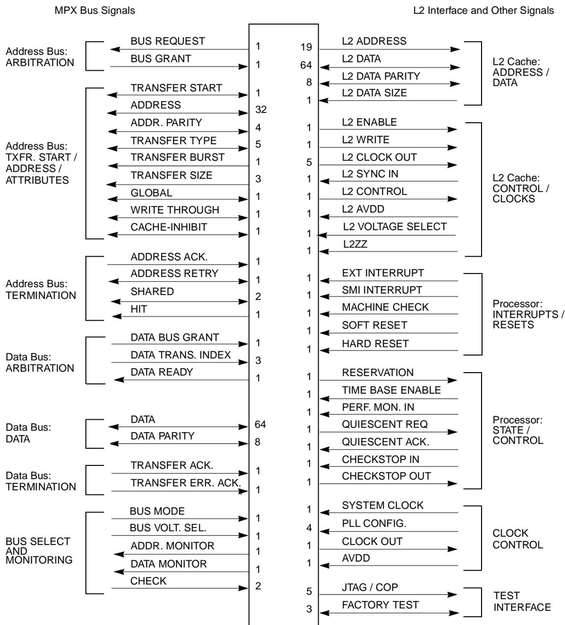
Note: 266 total signal pins are shown (including analog  $V_{DDs}$ )
