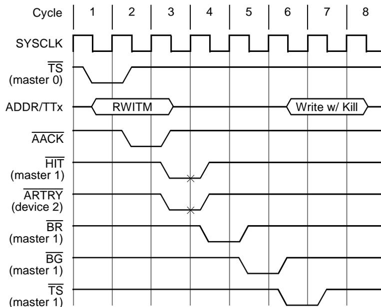
Cycle 3: Master 1 asserts  $\overline{\text{HIT}}$ , but device 2 retries the transaction.
