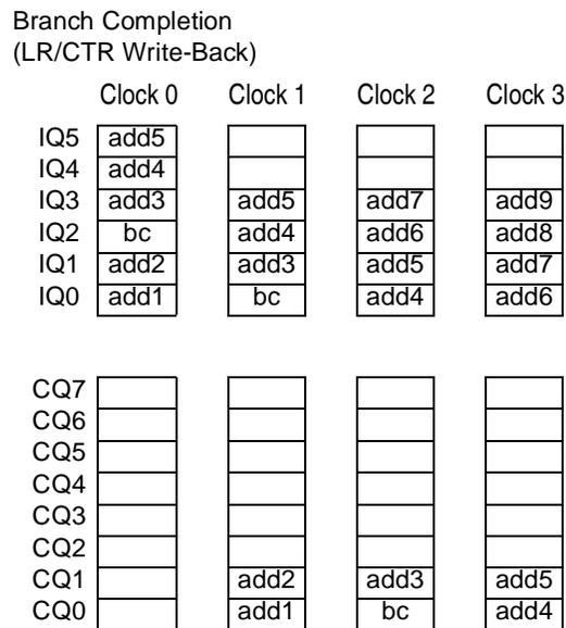
**Figure 6-13. Branch Completion**
