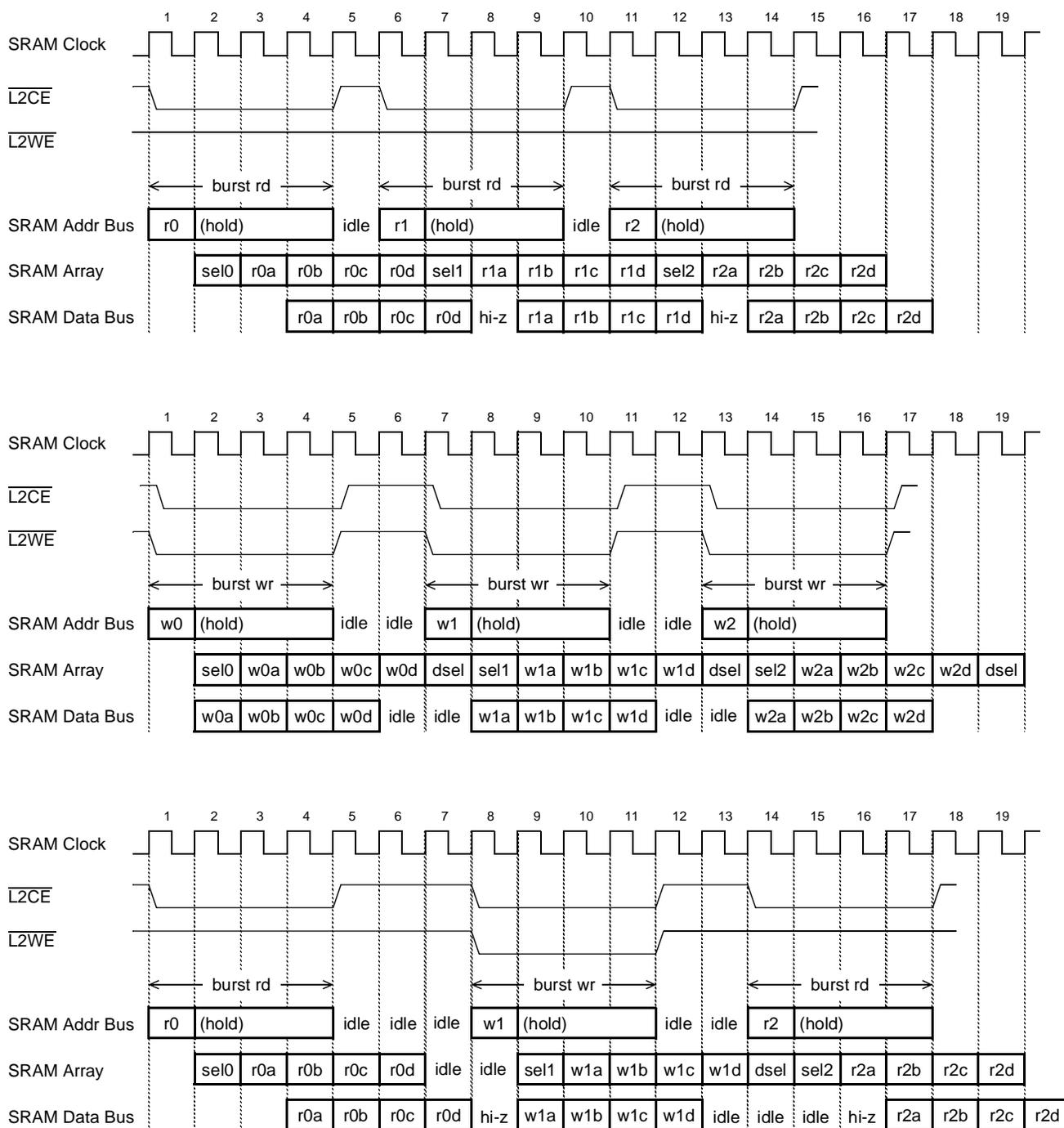
**Note:** For PB3, L2ZZ is reused as  $\overline{\text{L2ADS}}$  and asserts during the first clock only of each  $\overline{\text{L2CE}}$  assertion. For PB3, internal array access requires 1 cycle to row select, 1 cycle for each column select of burst (a-d), 1 cycle deselect if write.
