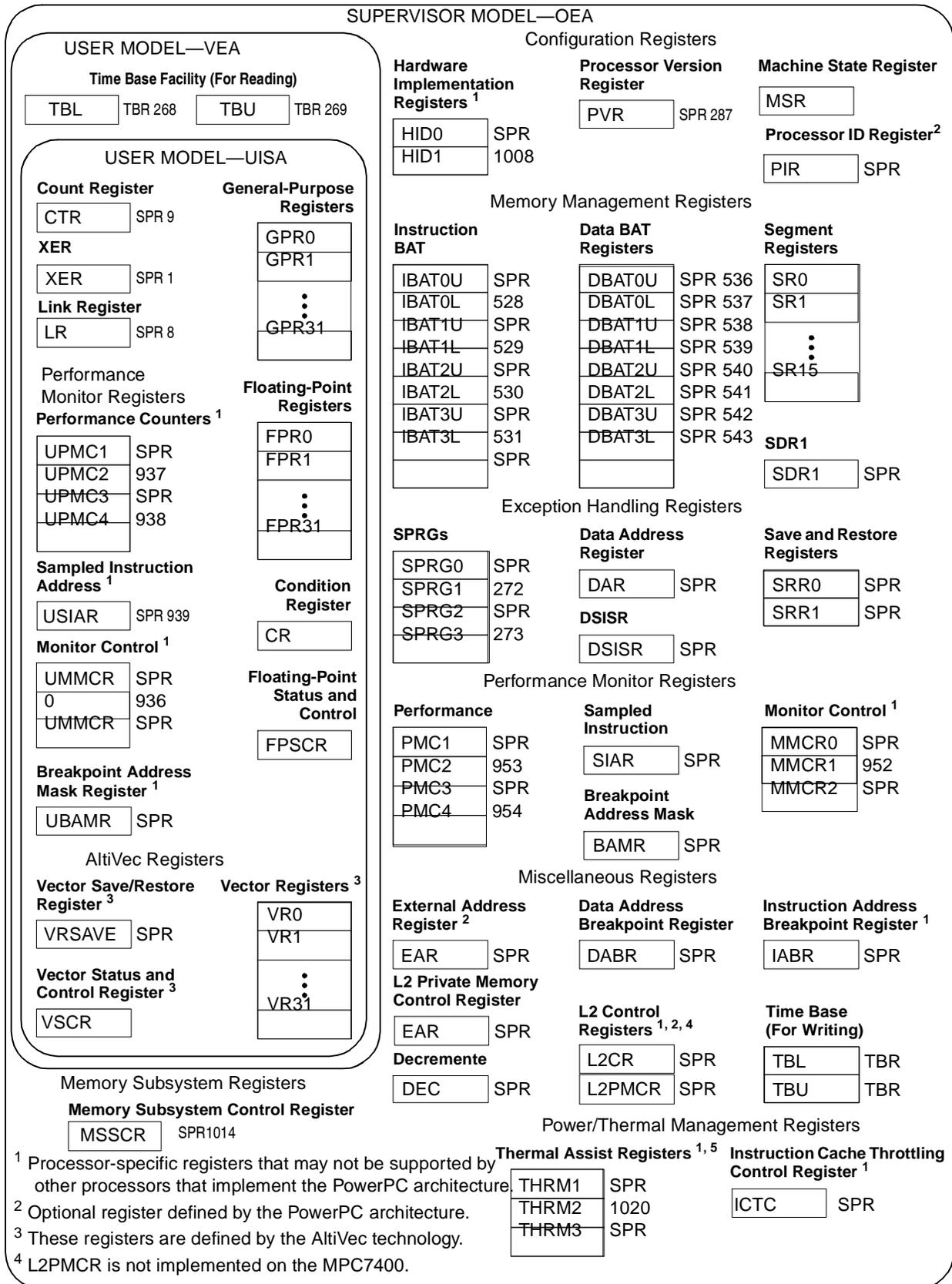
**Figure 1-5. MPC7410 Microprocessor Programming Model—Registers**
