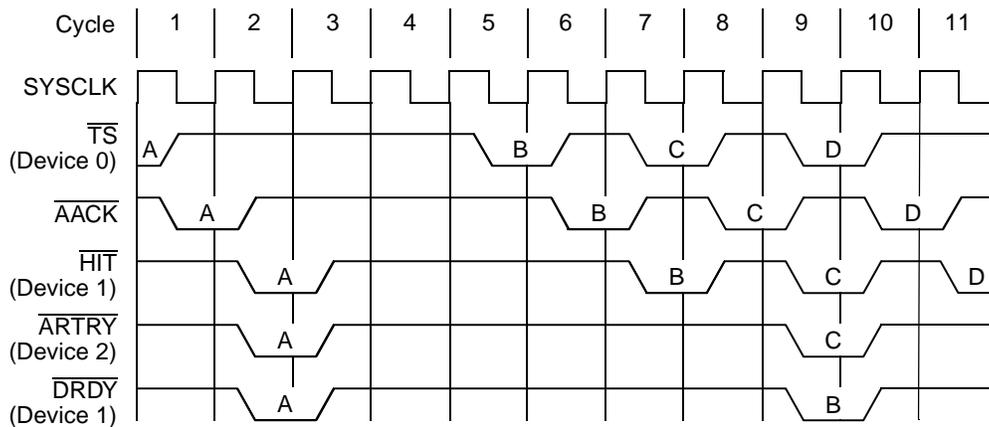
Cycle 2: Transaction A receives an  $\overline{\text{ARTRY}}$  so the  $\overline{\text{HIT}}$  and  $\overline{\text{DRDY}}$  signals are ignored by the system.
