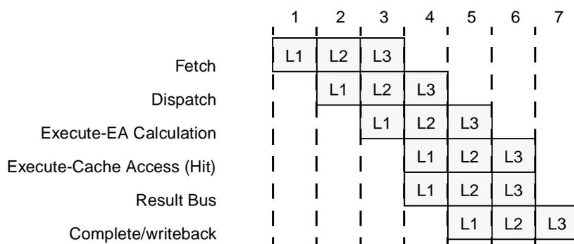
Figure 6-7. Data L1 Load Hit (No Stalls)
