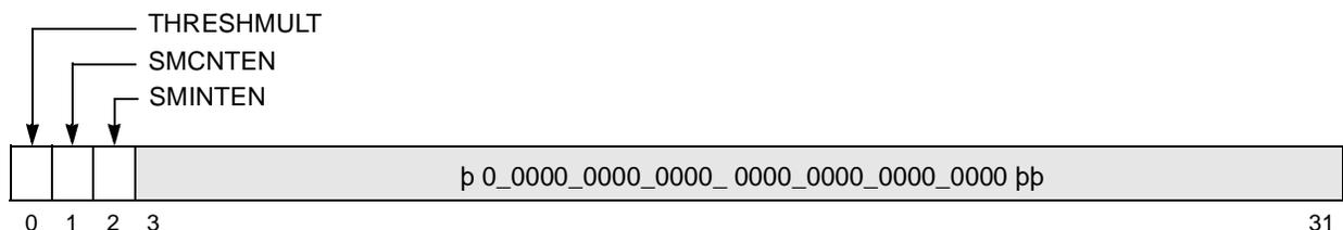
Figure 11-3. Monitor Mode Control Register 2 (MMCR2)
