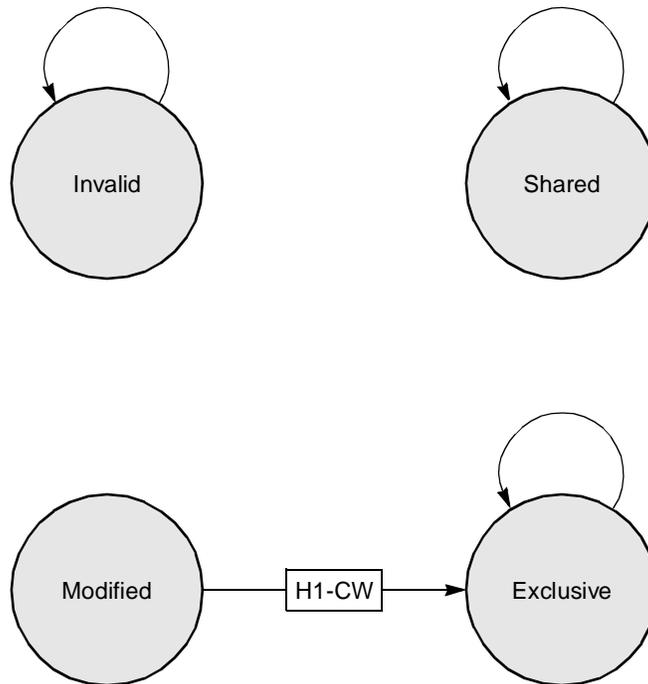
**Figure 3-17. Clean Transaction—MPX Bus Mode, L1\_INTVEN = 0b110**
