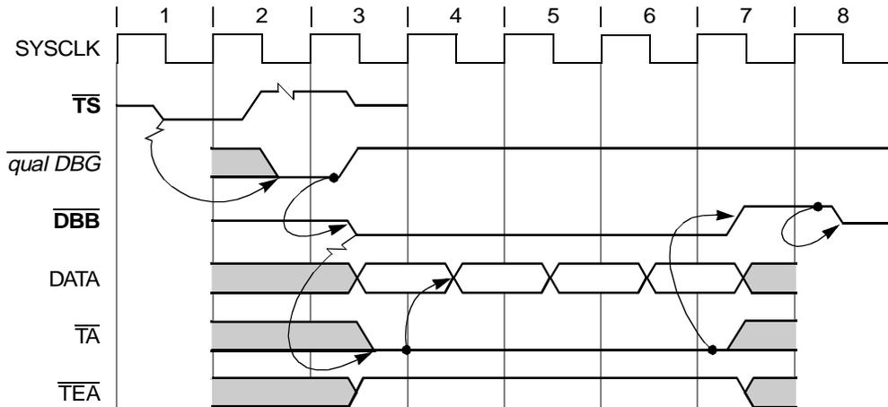
**Figure 9-10. Normal Burst Transaction**
