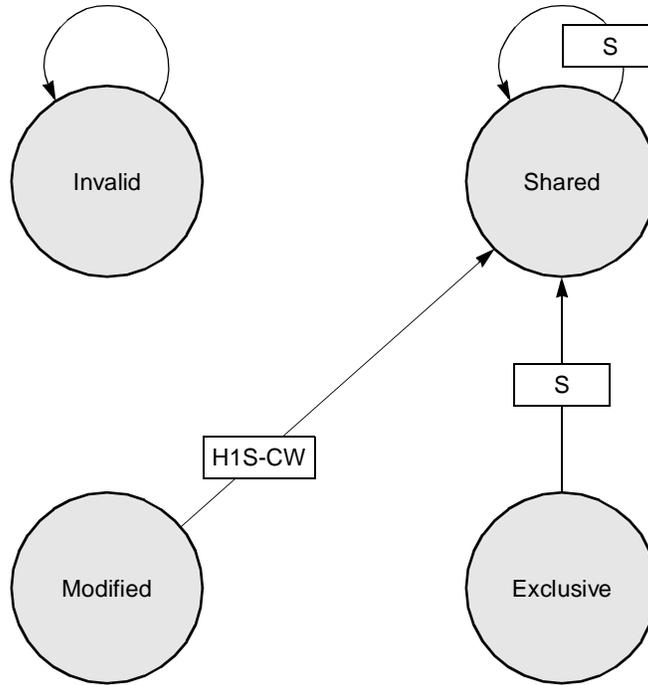
Figure 3-8. Read Transaction—MPX Bus Mode,  $L1\_INTVEN = 0b100$
