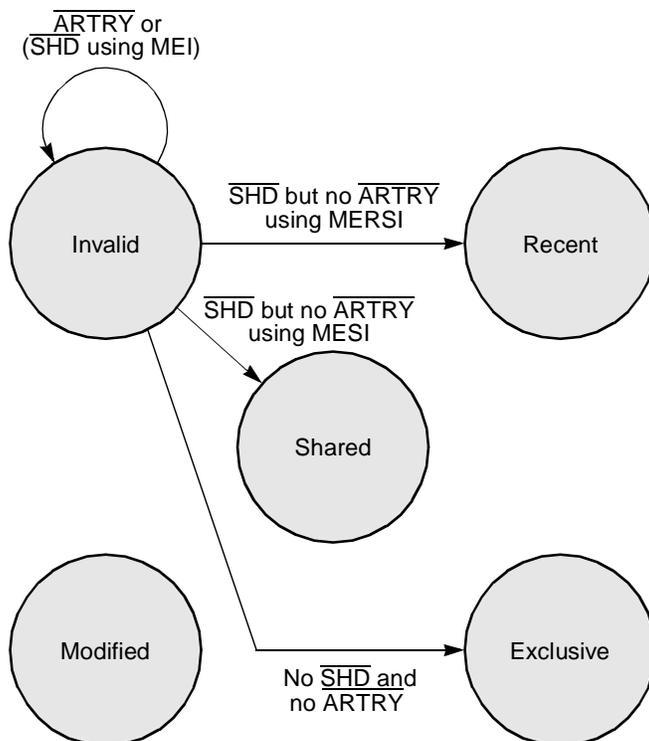
**Figure 3-31. Self-Generated Read (Caused by Instruction Fetch) Transaction**
