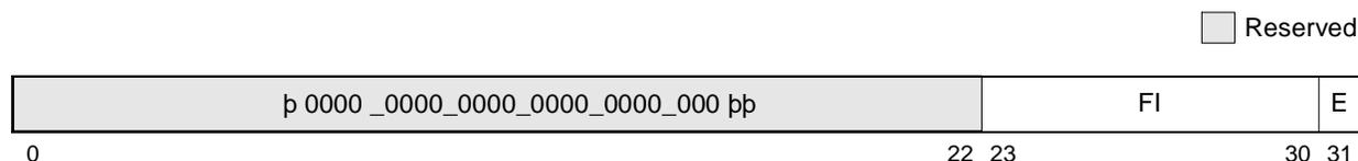
**Figure 2-11. Instruction Cache Throttling Control Register (ICTC)**
