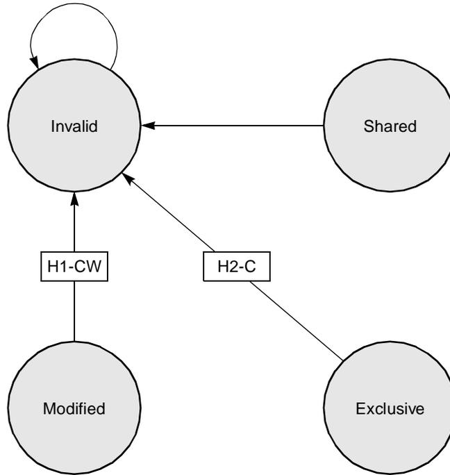
Figure 3-14. RWITM Transaction—MPX Bus Mode, L1\_INTVEN = 0b110
