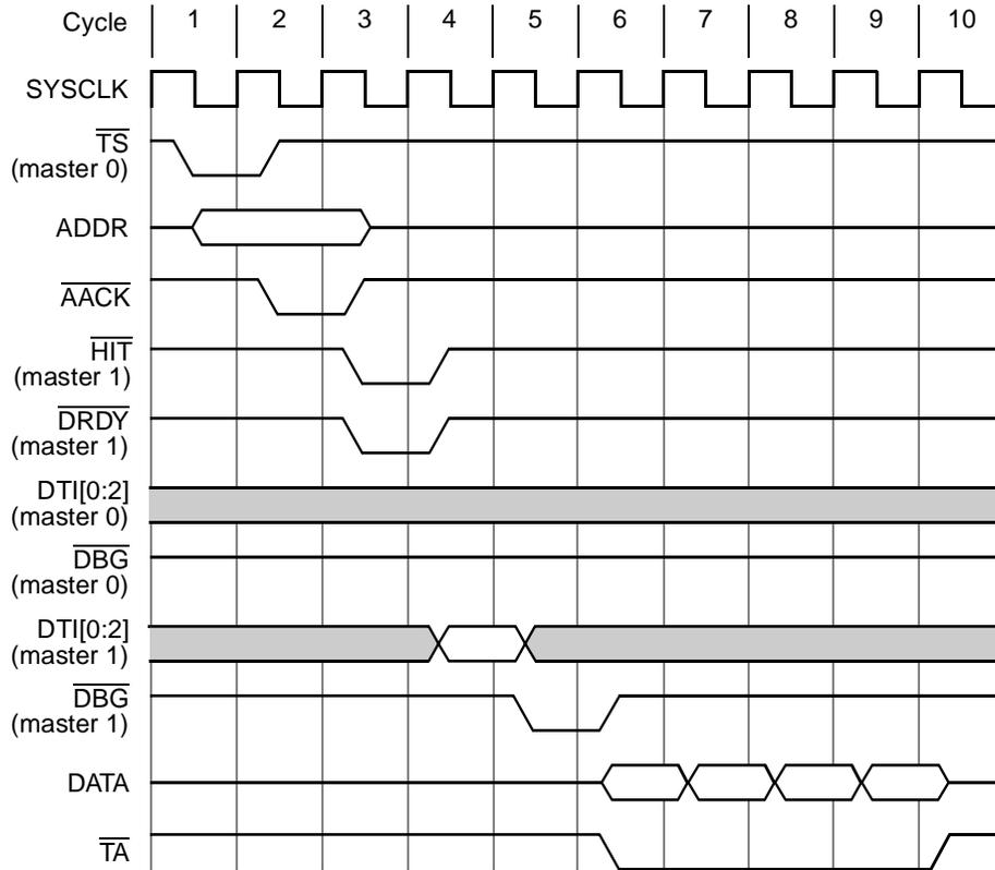
Figure 9-25. Data-Only Transaction for a Flush Operation
