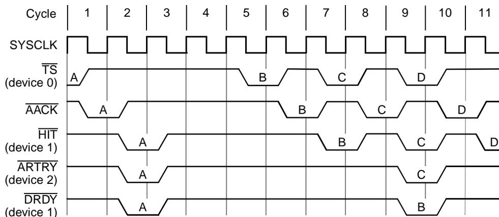
Cycle 3: Transaction A receives an  $\overline{\text{ARTRY}}$  so the  $\overline{\text{HIT}}$  and  $\overline{\text{DRDY}}$  signals are ignored by the system.
