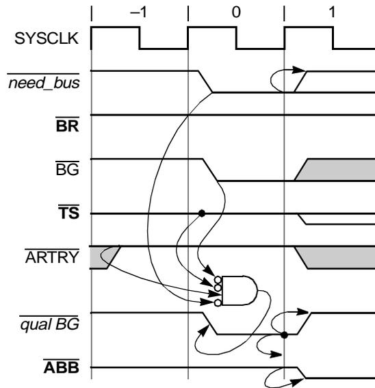
Figure 9-5. Address Bus Arbitration Showing Bus Parking
