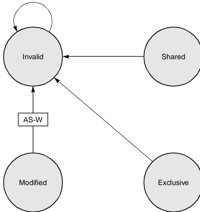
Figure 3-15. Write Transaction—MPX Bus Mode, L1\_INTVEN = 0b110
