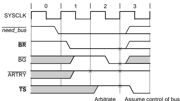
**Figure 9-18. MPX Bus Address Bus Arbitration—Non-Parked Case**
