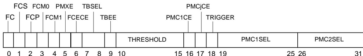
**Figure 2-12. Monitor Mode Control Register 0 (MMCR0)**
