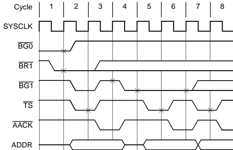
Cycle 1: Master 0 has a parked address bus grant. Master 0 has an address tenure ready and a qualified bus grant, so it queues an address tenure for the next cycle. Also in cycle 1, the arbiter samples a bus request from master 1, so the arbiter queues a switch of the bus grants from master 0 to master 1. The arbiter can safely do this, because the qualified bus grant equation for MPX bus masters includes  $\neg\overline{TS}$ .
