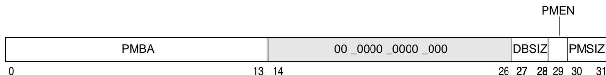
**Figure 2-6. L2 Private Memory Control Register (L2PMCR)—MPC7410 Only**
