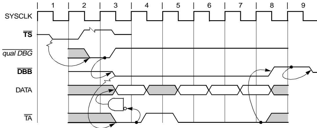
**Figure 9-11. Read Burst with  $\overline{TA}$  Wait States**
