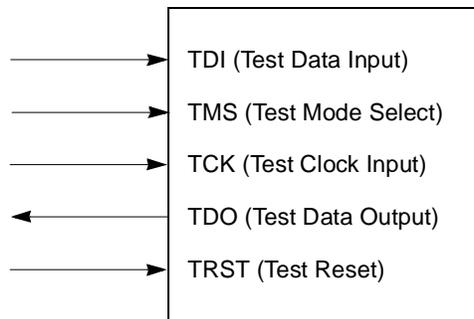
**Figure 9-28. IEEE Std. 1149.1a-1993 Compliant Boundary-Scan Interface**
