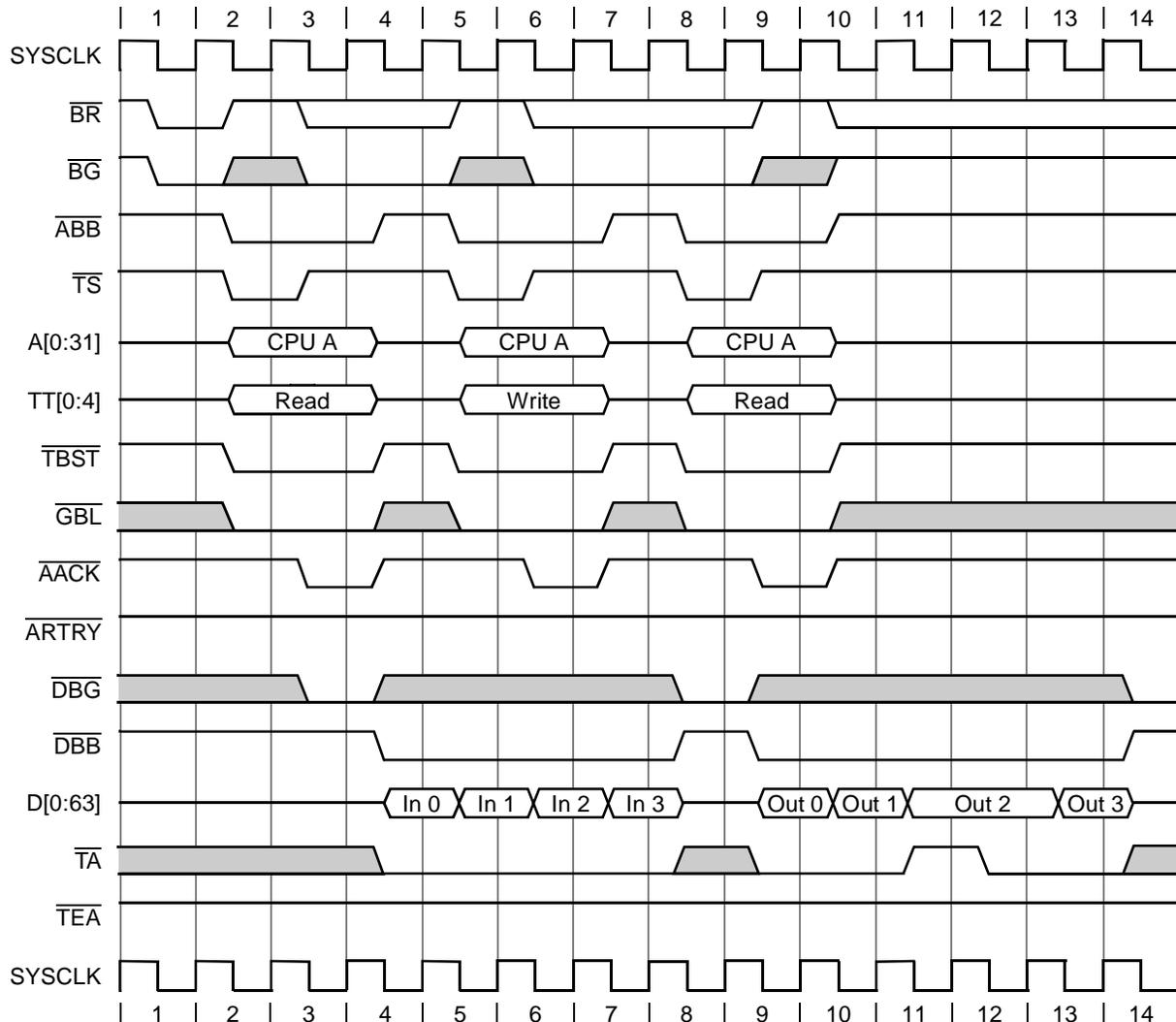
Figure 9-16. Burst Transfers with Data Delay Controls
