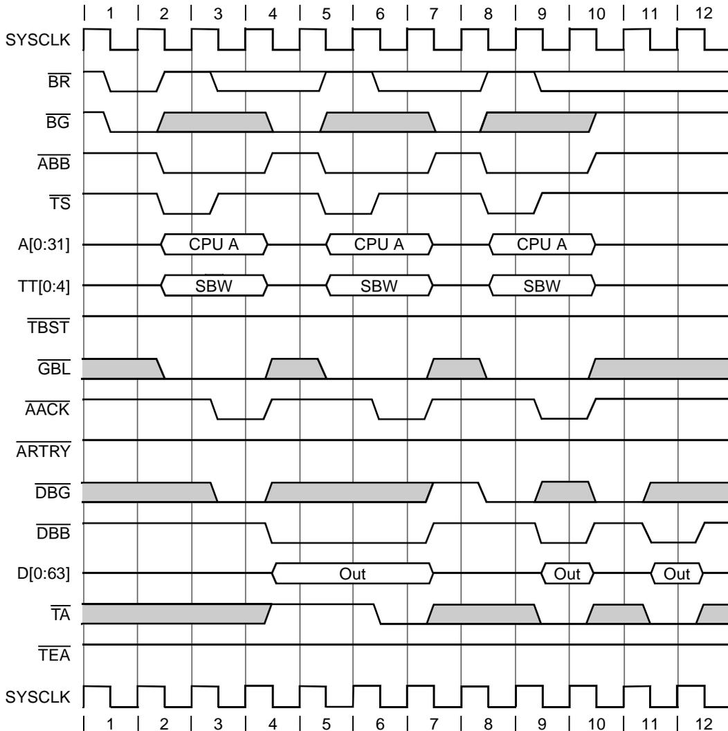
Figure 9-15. Single-Beat Writes Showing Data Delay Controls
