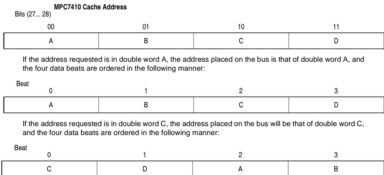
**Figure 3-39. Double-Word Address Ordering—Critical Double Word First**
