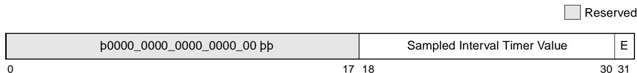
**Figure 2-10. Thermal Management Register 3 (THRM3)—MPC7400 Only**
