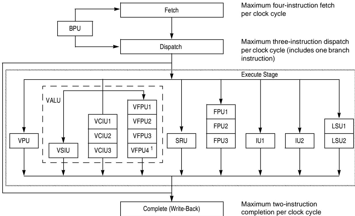
1 In non-Java mode, all VFPU instructions are pipelined as shown. In Java mode, all VFPU instructions need a fifth execution cycle; however, data forwarding for instruction dependency can still occur at the end of the fourth execution cycle as in non-Java mode.
