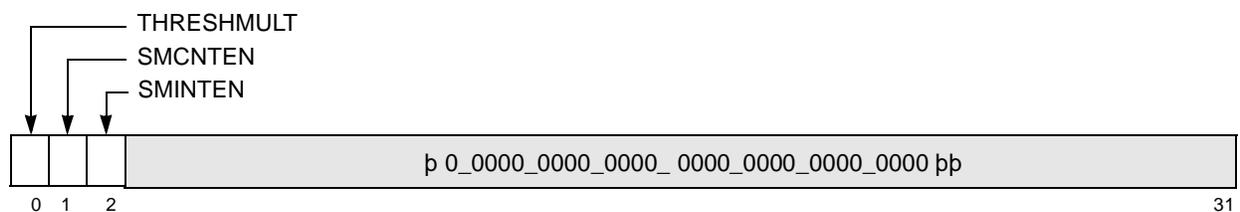
**Figure 2-14. Monitor Mode Control Register 2 (MMCR2)**
