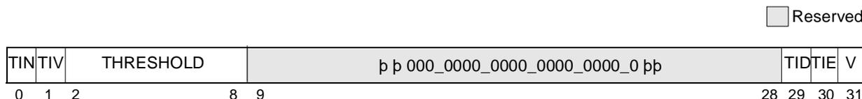
**Figure 2-9. Thermal Management Registers 1–2 (THRM1–THRM2)—MPC7400 Only**
