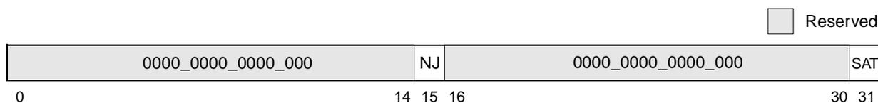
Figure 7-2. Vector Status and Control Register (VSCR)
