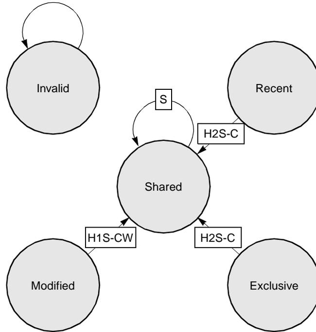
**Figure 3-19. Read Transaction—MPX Bus Mode, L1\_INTVEN = 0b111**
