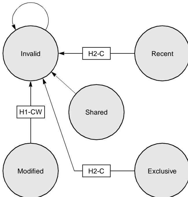
Figure 3-20. RWITM Transaction—MPX Bus Mode, L1\_INTVEN = 0b111
