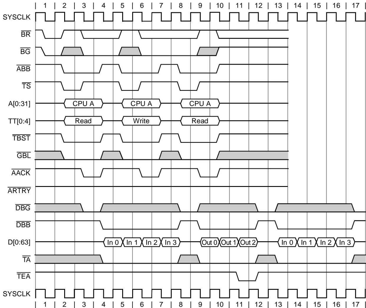
Figure 9-17. Use of Transfer Error Acknowledge ( $\overline{\text{TEA}}$ )
