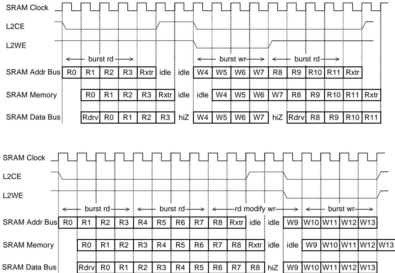
**Notes:** Rdrv indicates where some burst RAMs may begin driving the data bus. Rxtr indicates where an extra read cycle is signaled to keep the burst RAM driving the data bus for the last read. The MPC7410 does not support aborted reads
