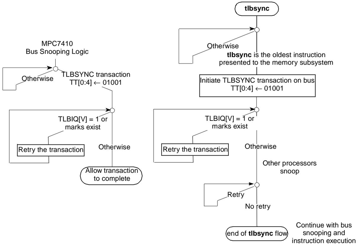
Figure 5-9. **tlbsync** Instruction Execution and Bus Snooping Flow
