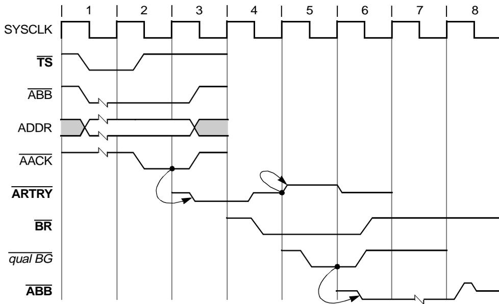
Figure 9-7. Snooped Address Cycle with  $\overline{\text{ARTRY}}$
