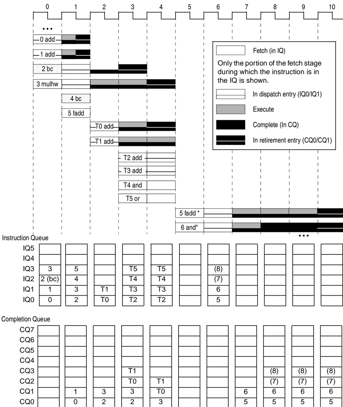
\* Instructions 5 and 6 are not in the IQ in clock cycle 5. Here, the fetch stage shows cache latency.
