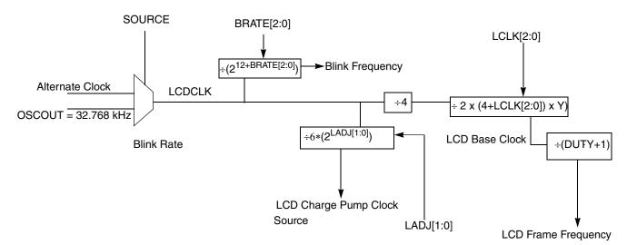
Figure 13-12. LCD Clock Tree
