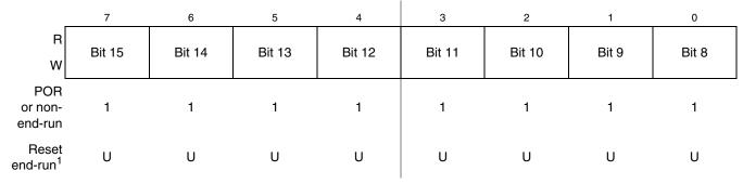
Figure 19-2. Debug Comparator A High Register (DBGCAH)
