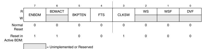
Figure 18-5. BDC Status and Control Register (BDCSCR)
