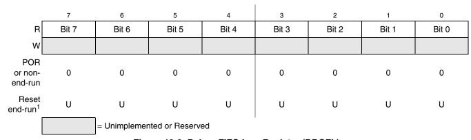
Figure 19-9. Debug FIFO Low Register (DBGFL)
