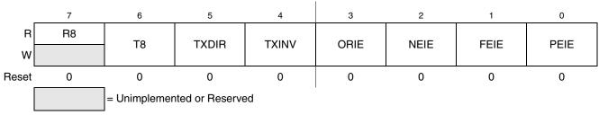
Figure 14-10. SCI Control Register 3 (SCIC3)
