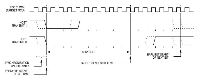
Figure 18-2. BDC Host-to-Target Serial Bit Timing
