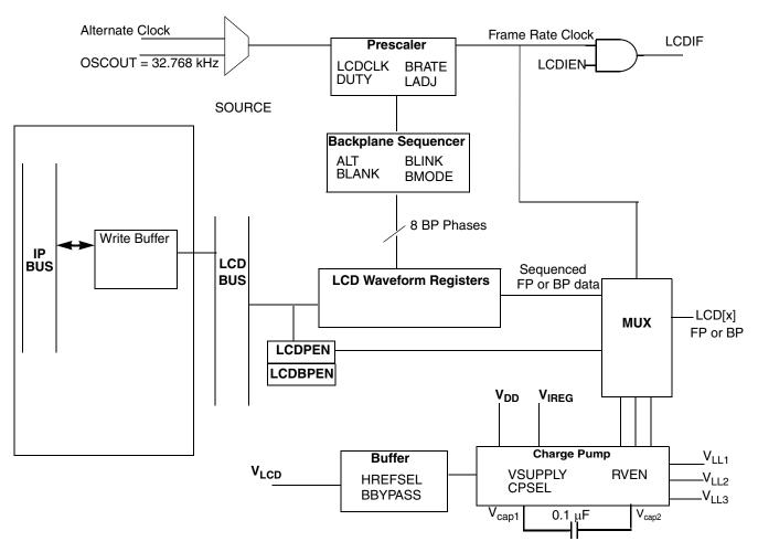
Figure 13-2. LCD Driver Block Diagram
