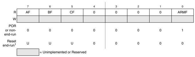
Figure 19-15. Debug Status Register (DBGS)
