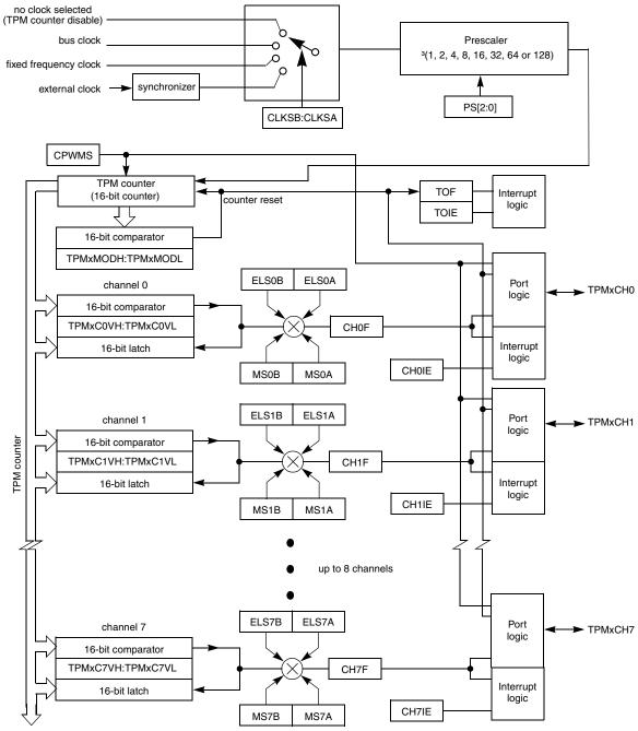
Figure 16-2. TPM Block Diagram
