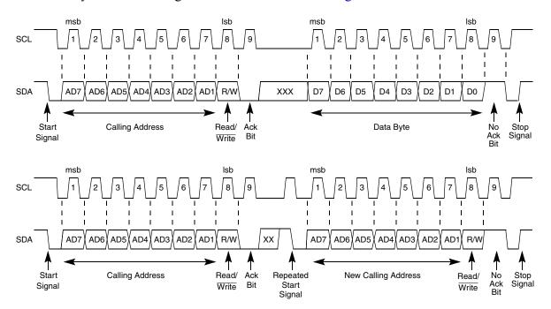
Figure 12-9. IIC Bus Transmission Signals
