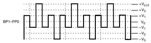
Figure 13-20. "f" Segment Voltage Waveform
