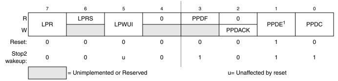
Figure 5-10. System Power Management Status and Control 2 Register (SPMSC2)
