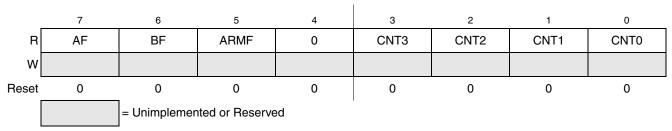
Figure 18-9. Debug Status Register (DBGS)
