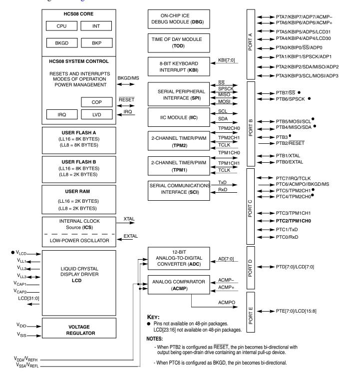
Figure 1-1. MC9S08LL16 Series Block Diagram
