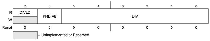
Figure 4-5. FLASH Clock Divider Register (FCDIV)
