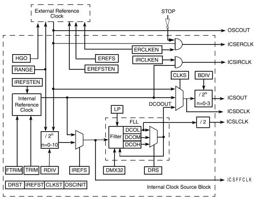
Figure 11-2. Internal Clock Source (ICS) Block Diagram
