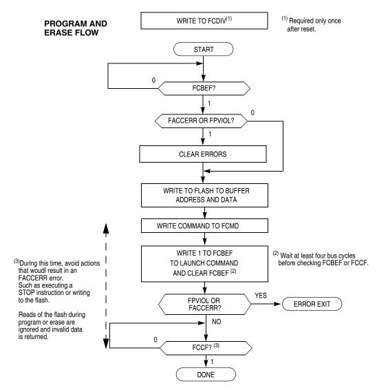
Figure 4-2. FLASH Program and Erase Flowchart
