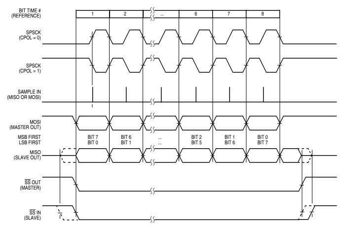
Figure 15-11. SPI Clock Formats (CPHA = 0)
