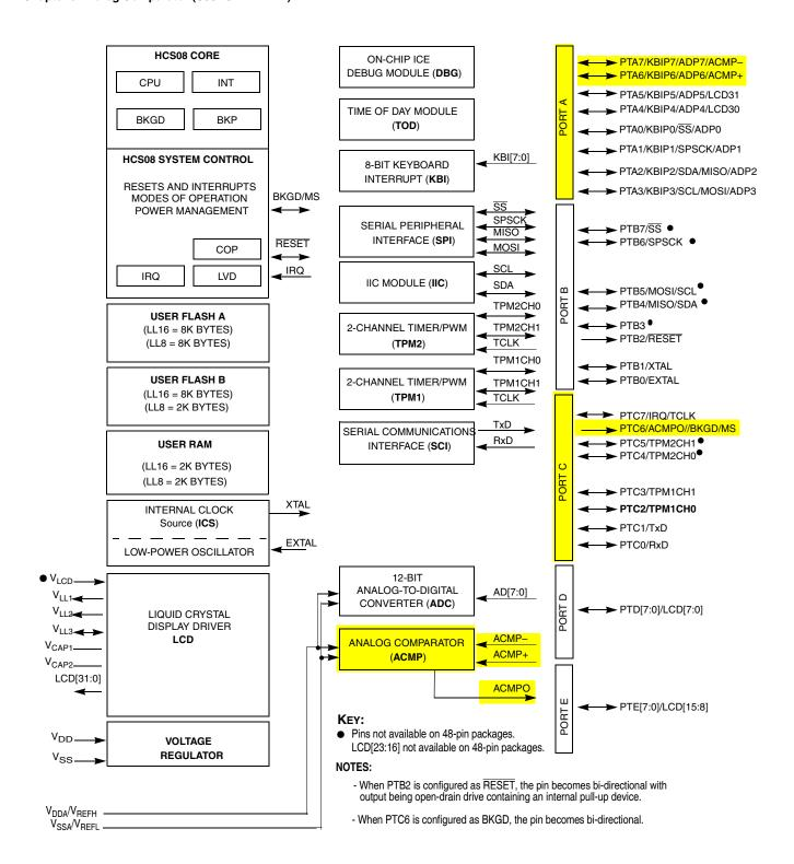
Figure 9-1. MC9S08LL16 Series Block Diagram Highlighting ACMP Block and Pins
