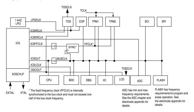
Figure 1-2. System Clock Distribution Diagram
