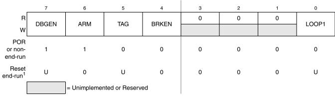
Figure 19-13. Debug Control Register (DBGC)
