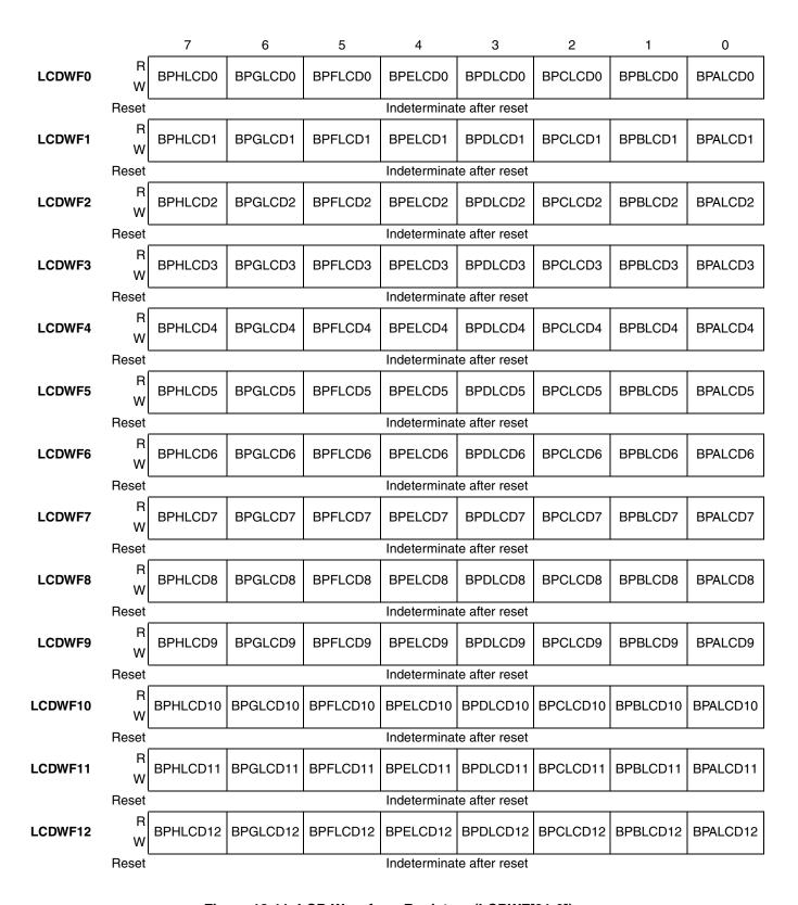
Figure 13-11. LCD Waveform Registers (LCDWF[31:0])
