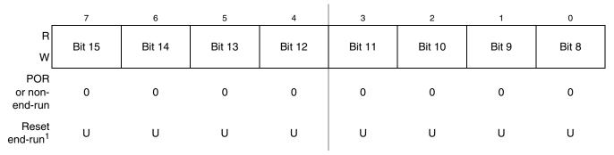
Figure 19-4. Debug Comparator B High Register (DBGCBH)
