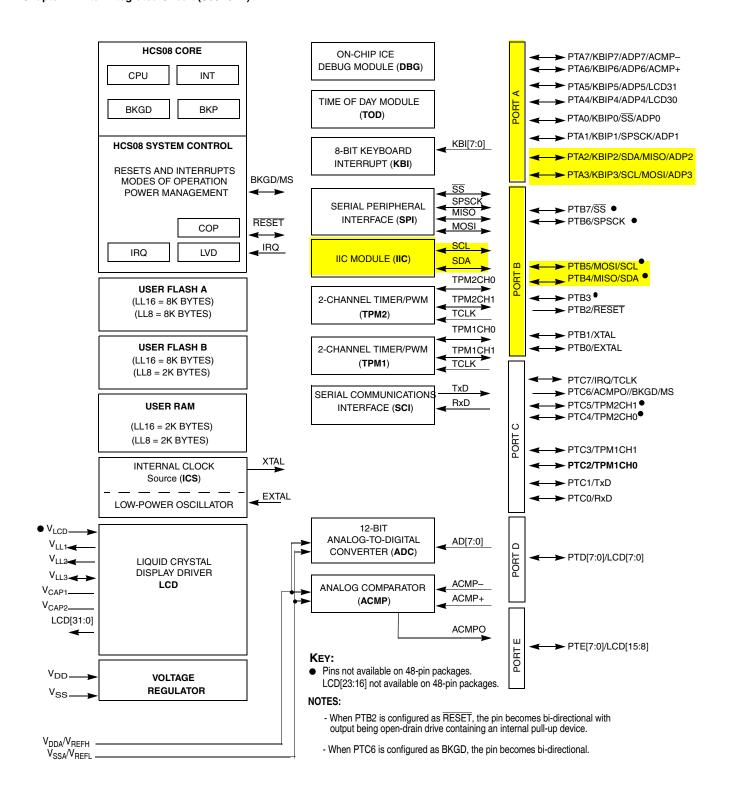
Figure 12-1. MC9S08LL16 Series Block Diagram Highlighting the IIC Block and Pins
