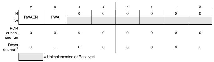
Figure 19-10. Debug Comparator A Extension Register (DBGCAX)
