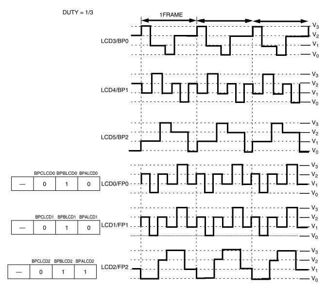
Figure 13-19. LCD Waveforms
