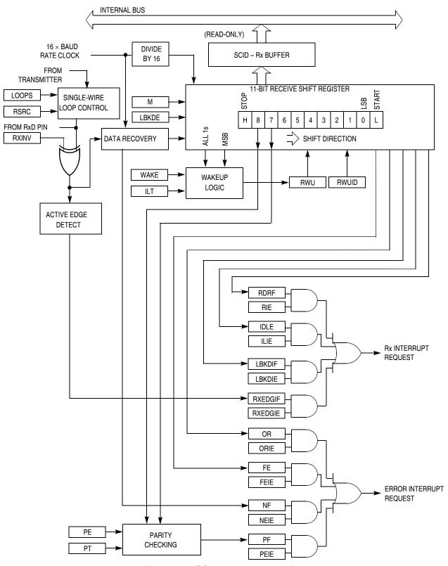
Figure 14-3. SCI Receiver Block Diagram
