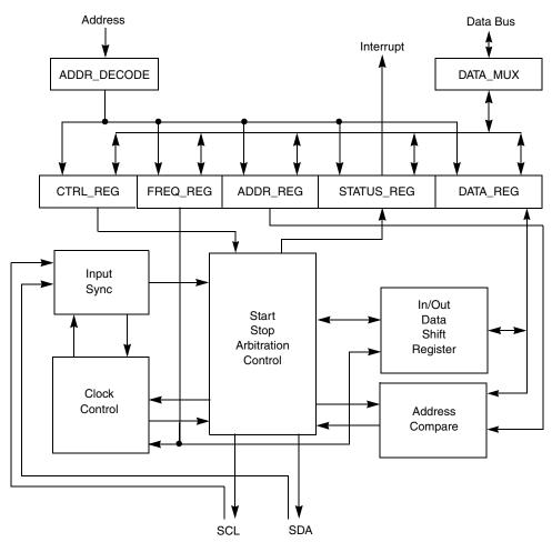
Figure 12-2. IIC Functional Block Diagram
