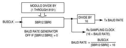
Figure 14-12. SCI Baud Rate Generation
