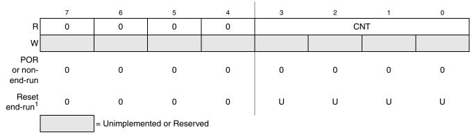
Figure 19-16. Debug Count Status Register (DBGCNT)
