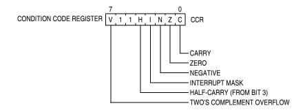
Figure 8-2. Condition Code Register
