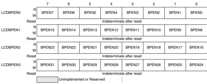
Figure 13-10. Backplane Enable Registers 0-3 (LCDBPEN0-LCDBPEN3)
