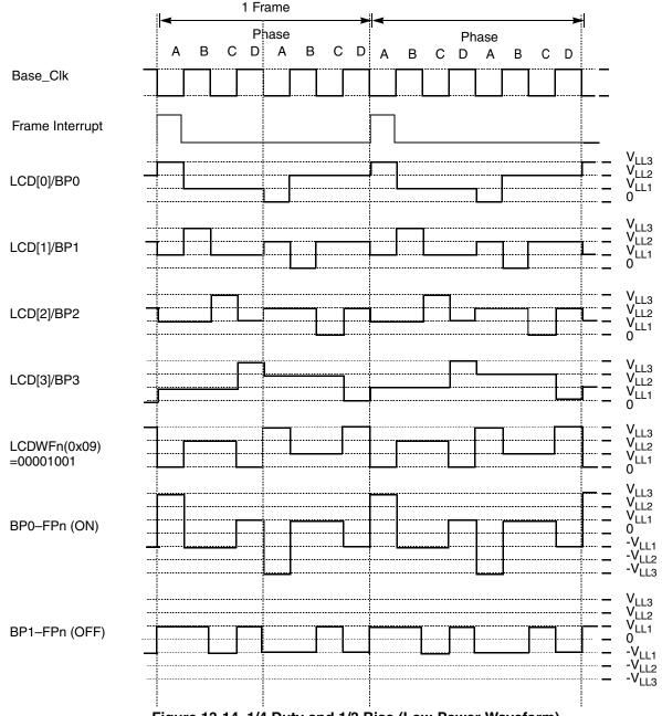
Figure 13-14. 1/4 Duty and 1/3 Bias (Low-Power Waveform)
