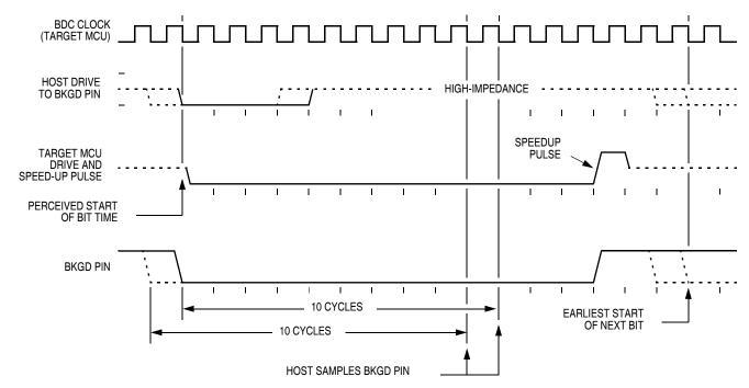
Figure 18-4. BDM Target-to-Host Serial Bit Timing (Logic 0)
