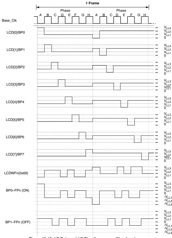
Figure 13-15. 1/8 Duty and 1/3 Bias (Low-power Waveform)
