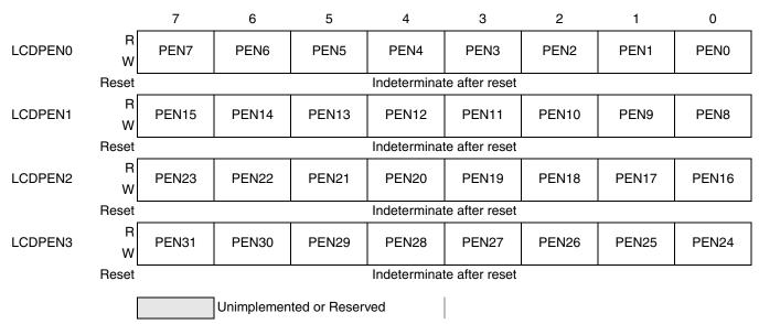
Figure 13-9. LCD Pin Enable Registers 0-3 (LCDPEN0-LCDPEN3)
