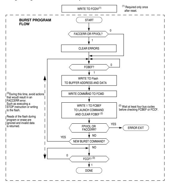
Figure 4-3. FLASH Burst Program Flowchart
