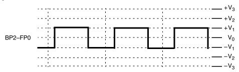
Figure 13-21. "e" Segment Voltage Waveform
