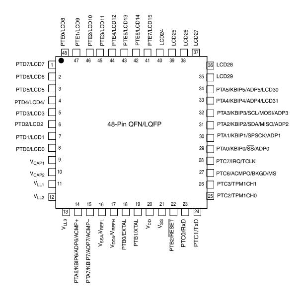
Note: V<sub>REFH</sub>/V<sub>REFL</sub> are internally connected to V<sub>DDA</sub>/V<sub>SSA</sub>
