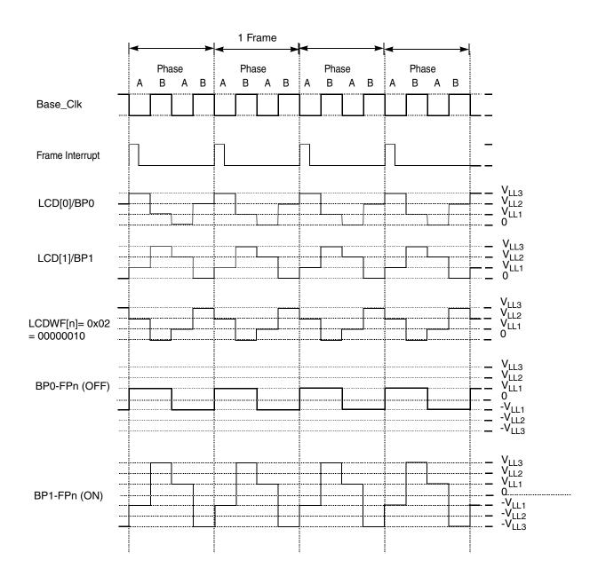
Figure 13-13. 1/2 Duty and 1/3 Bias (Low-Power Waveform)
