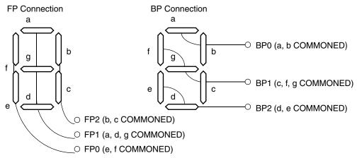
The above segment assignments are provided by the specification for the LCD glass for this example. For this LCD Module any of the LCD pins can be configured to be Frontplane 0-2 or Backplane 0-2. For this example we will set LCD[0] as FP0, LCD[1] as FP1, and LCD[2] as FP2. For this example we will set LCD[3] as BP0, LCD[4] as BP1 and LCD[5] as BP2.
