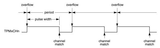
Figure 16-15. EPWM period and pulse width (ELSnA=0)
