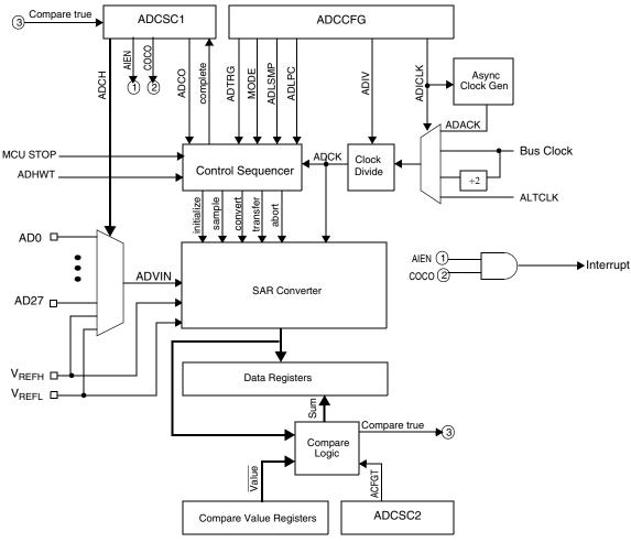
Figure 10-2. ADC Block Diagram
