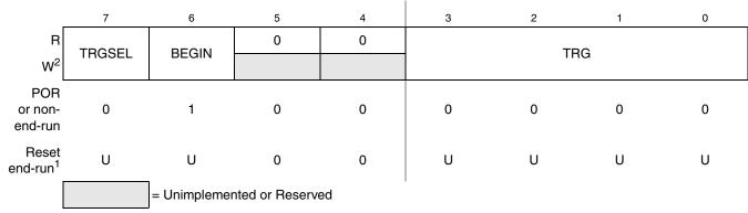
Figure 19-14. Debug Trigger Register (DBGT)
