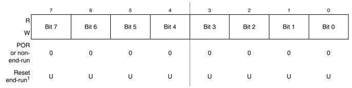
Figure 19-7. Debug Comparator C Low Register (DBGCCL)
