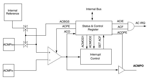
Figure 9-2. Analog Comparator Module Block Diagram
