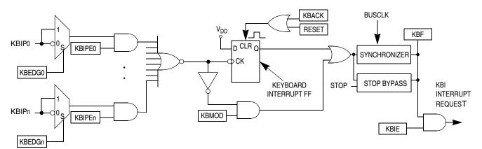
Figure 7-2. Keyboard Interrupt (KBI) Block Diagram
