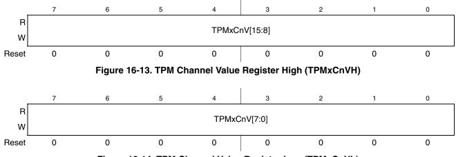
Figure 16-14. TPM Channel Value Register Low (TPMxCnVL)
