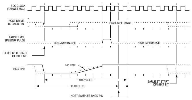
Figure 18-3. BDC Target-to-Host Serial Bit Timing (Logic 1)
