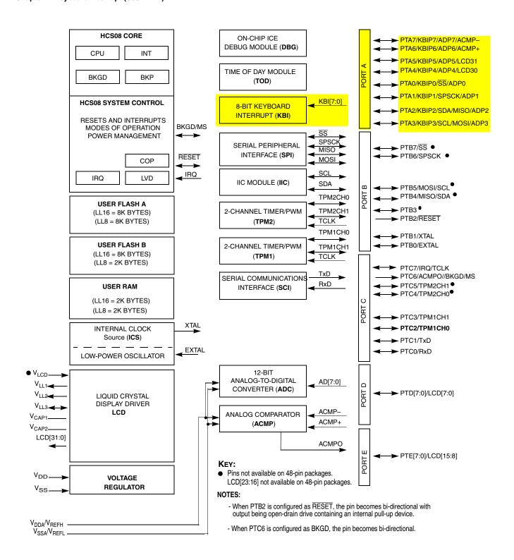
Figure 7-1. MC9S08LL16 Series Block Diagram Highlighting KBI Blocks
