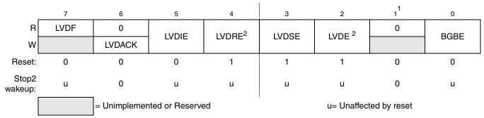
Figure 5-9. System Power Management Status and Control 1 Register (SPMSC1)
