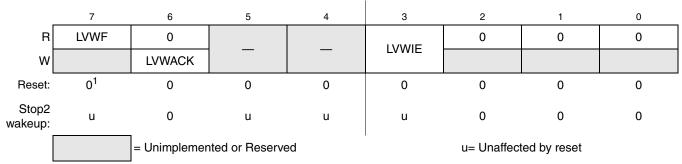
Figure 5-11. System Power Management Status and Control 3 Register (SPMSC3)
