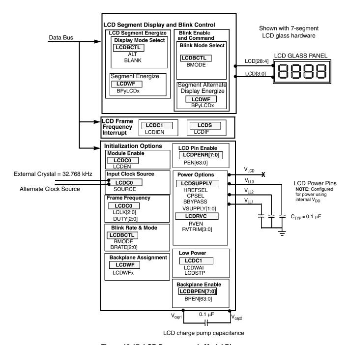
Figure 13-17. LCD Programmer's Model Diagram
