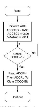
Figure 10-13. Initialization Flowchart for Example
