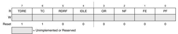
Figure 14-8. SCI Status Register 1 (SCIS1)
