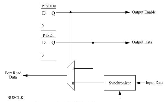
Figure 6-1. Parallel I/O Block Diagram
