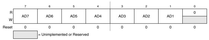
Figure 12-3. IIC Address Register (IICA)
