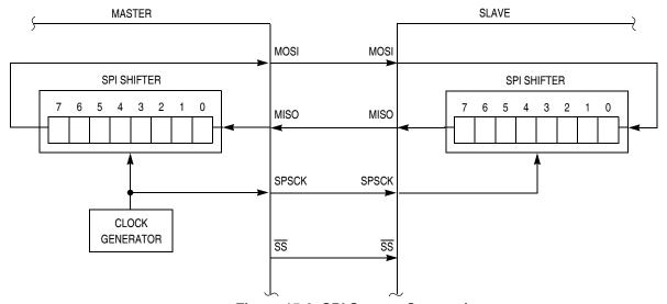
Figure 15-2. SPI System Connections
