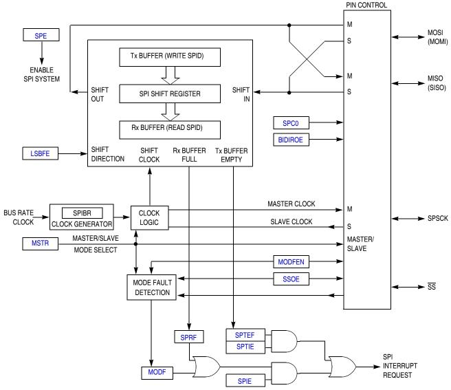
Figure 15-3. SPI Module Block Diagram
