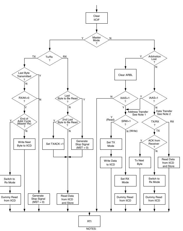
1. If general call is enabled, a check must be done to determine whether the received address was a general call address (0x00). If the received address was a general call address, then the general call must be handled by user software.
