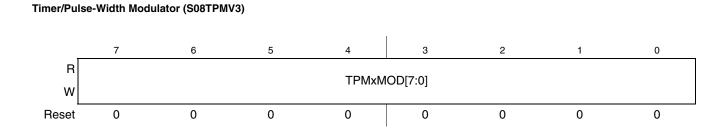
Reset the TPM counter before writing to the TPM modulo registers to avoid confusion about when the first counter overflow occurs.
