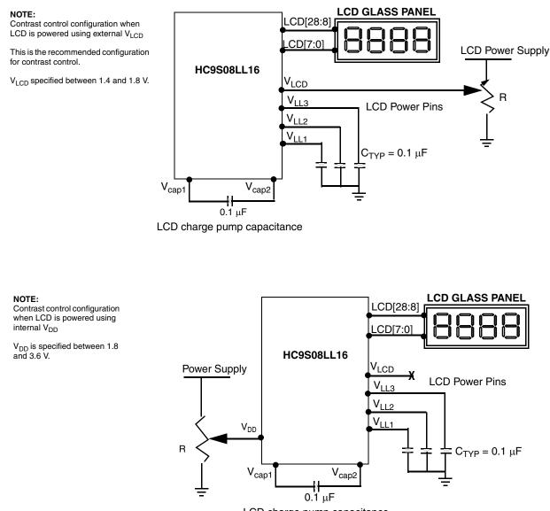
LCD charge pump capacitance
