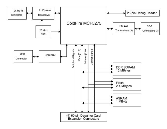
Figure 1-1. M5275EVB block diagram
