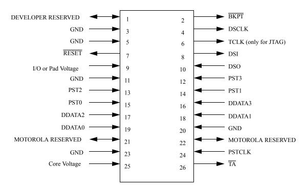
Figure 1-4. J1- BDM Connector pin assignment
