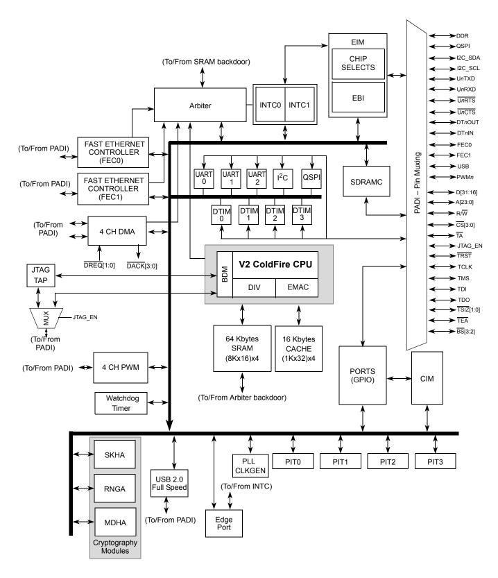
Figure 1-2. MCF5275 Block Diagram
