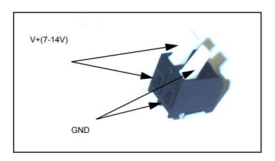
Figure 2-3. 2-Lever Power Connector
