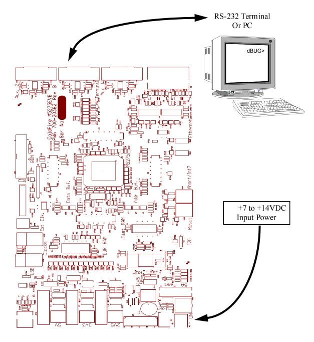
Figure 2-1. Minimum System Configuration
