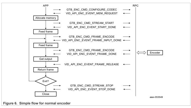
The input frame buffer is set through the buffer descriptor: pSharedInterface -> pEncCtrlInterface [str idx] ->pEncYUVBufferDesc.
