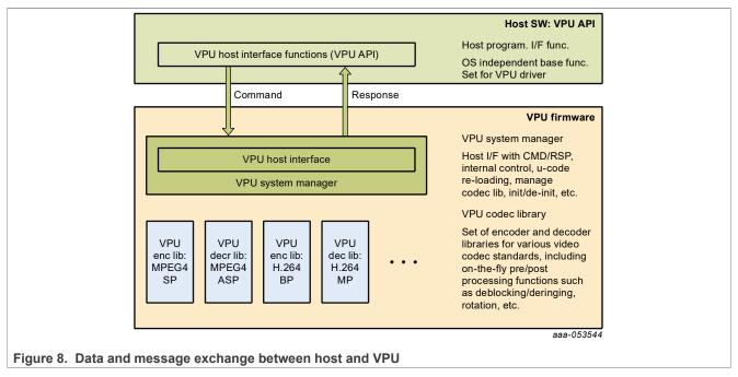
All bitstream and picture data is accessed directly by the host processor and VPU. The related information about the data transfer, command, and responses is exchanged through the host interface. The host interface
