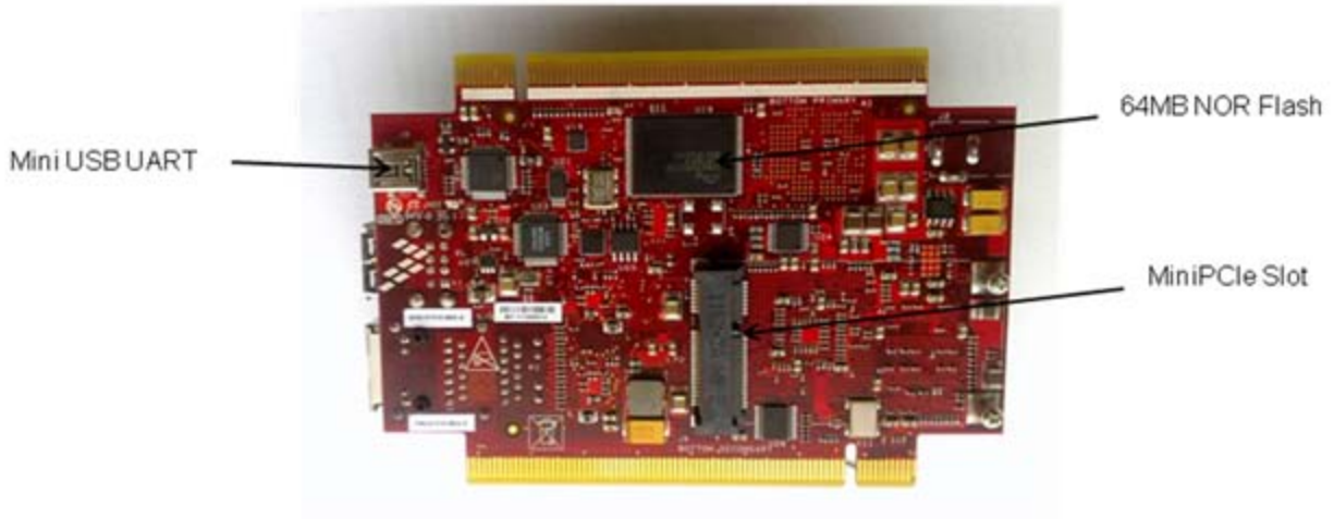
Figure 2-3: Secondary Side Main Features
