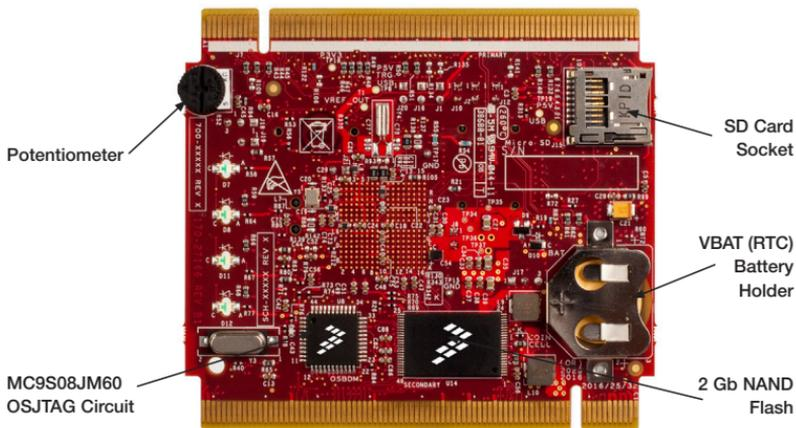
**Figure 2:** Back side of TWR-K70F120M module.
