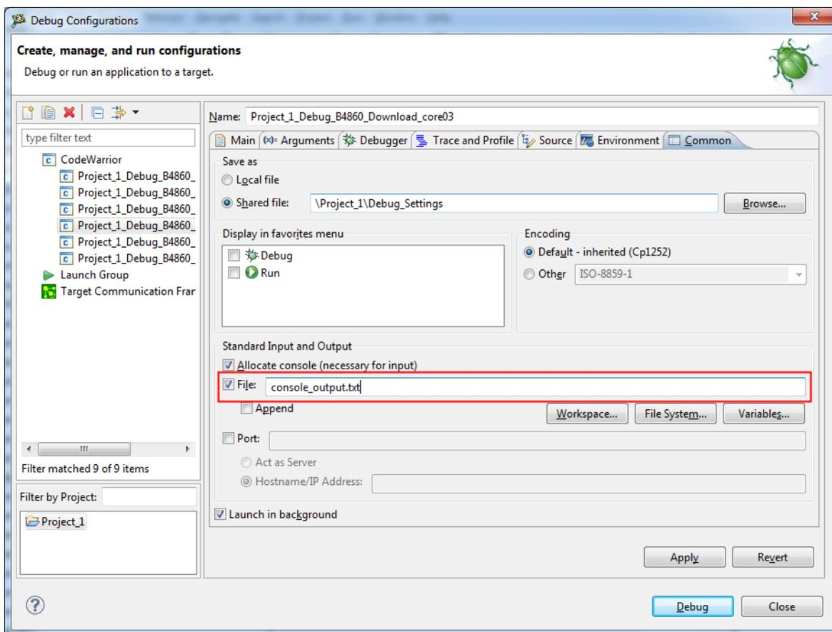
Figure 7-25. Debug Configurations-Common Page
