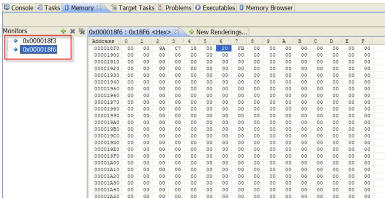
**Figure 7-12. Memory View with Multiple Addresses**
